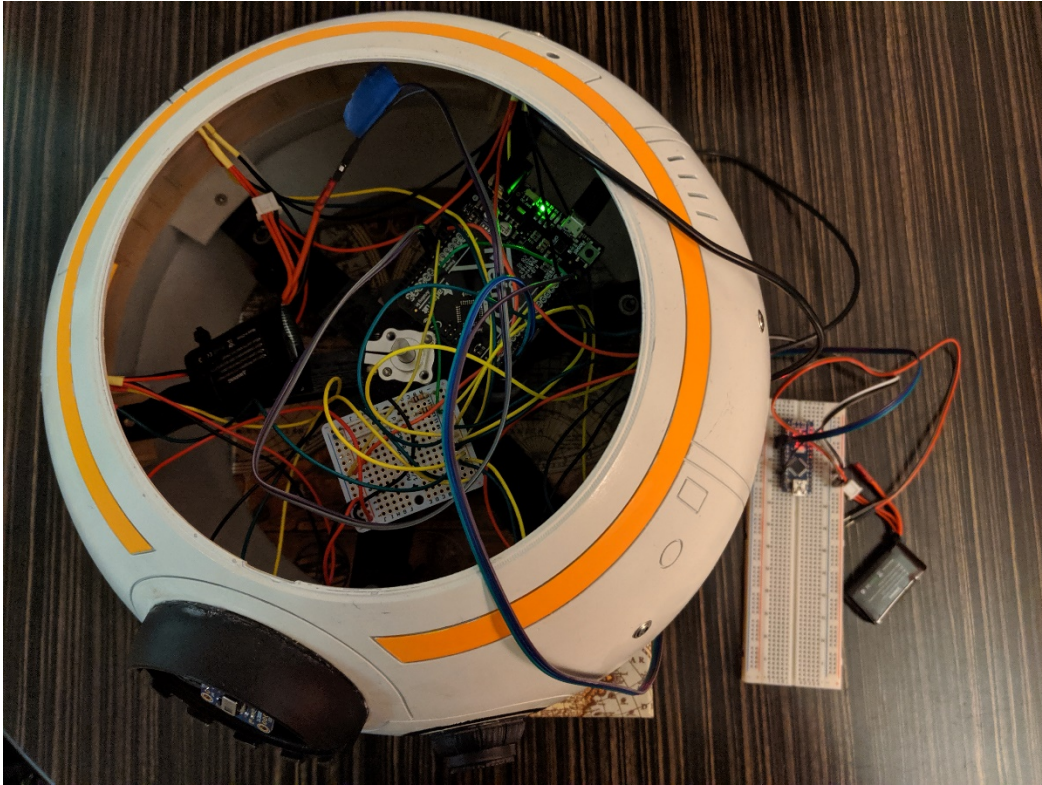
Figure 15 Sensors Wired in Dome
