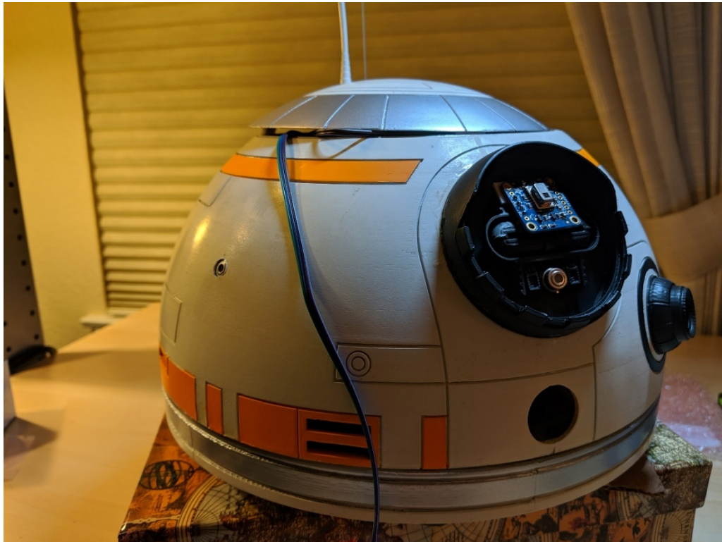
Image of Sensor Placement in Dome
