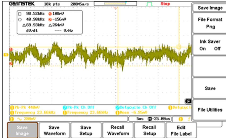
Figure 5.7: Output ripple of the 12V converter
