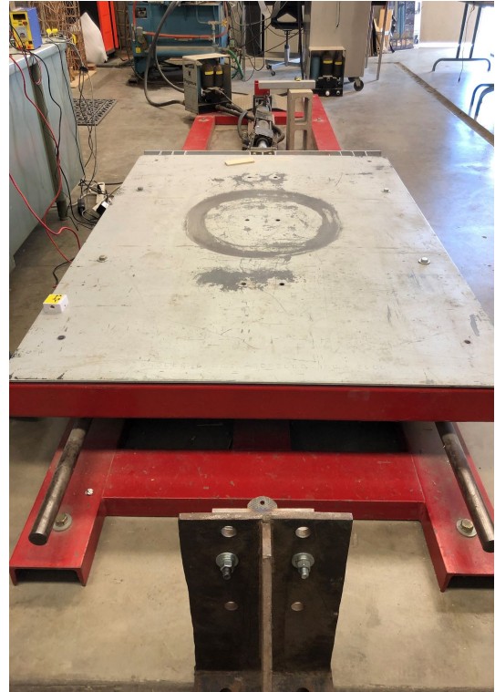
Figure 3.1.1 The shake table in the seismic lab.
