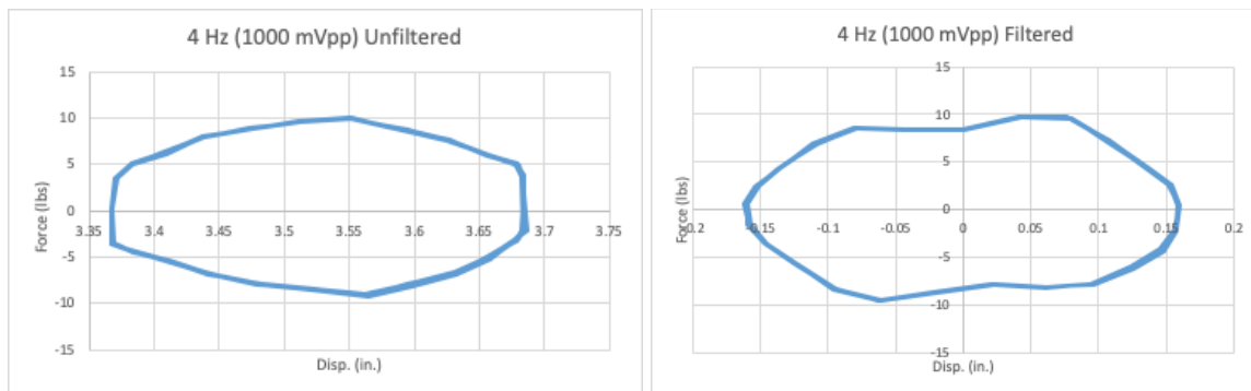
Figure 4.3 Hysteric Curve at 4 Hz and 1000 mVpp for filtered and unfiltered data.
