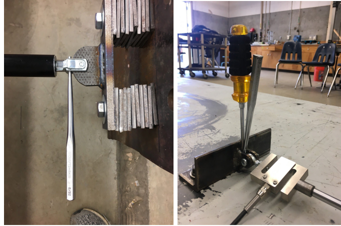
Figure 3.2.2 Detailed image of placement of pinned connection of damper to angled base plate with inserted tools.
