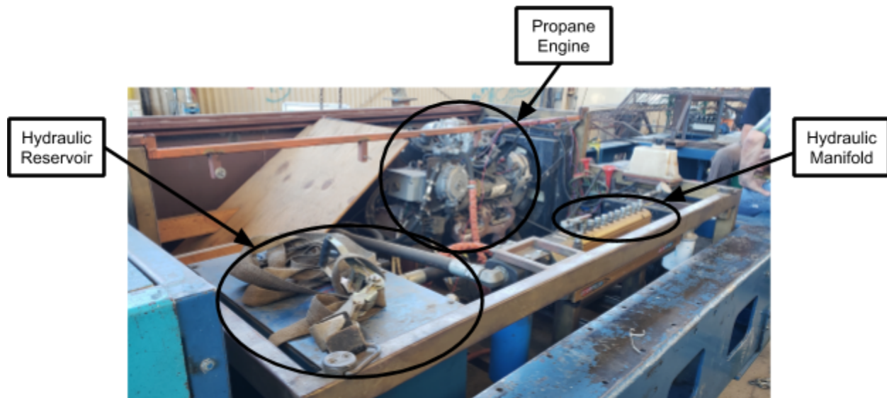
Figure 2. The Current Rose Float Animation System
