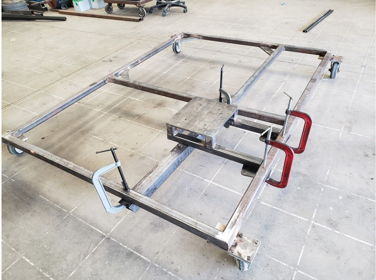
Figure 8. Motor Mount Installation on Lower Half System Frame
