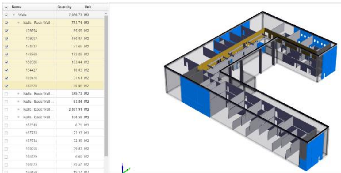
Figure 6 Assemble QTO of Masonry Walls, Highlighted Blue
