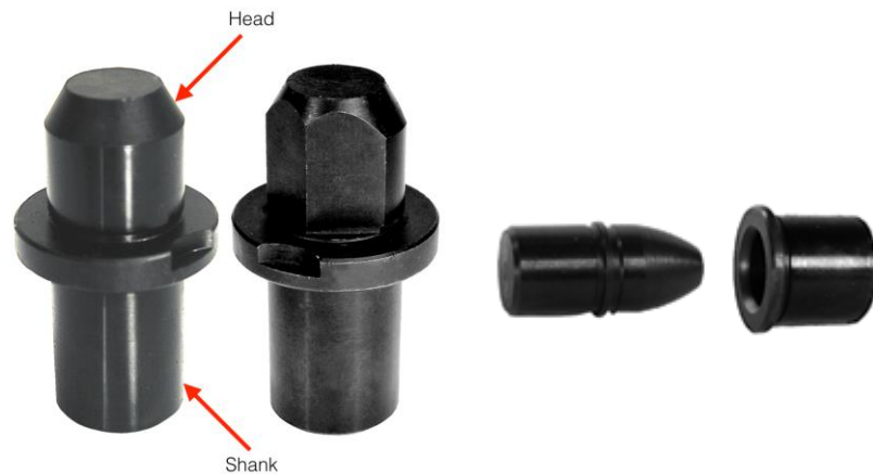
Figure 19 Carrlane locating pins. Head and shank are concentric to within 0.0005".
