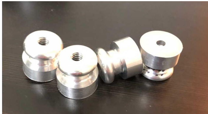
Figure 36. Adjustment screws. By turning these, the slides will move back and forth within their mounts.
