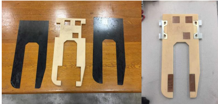
Figure 38. Individual drivetrain plate parts being test fitted.
