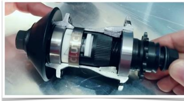
Figure 12 Odyssey conical clutched hub cut away
