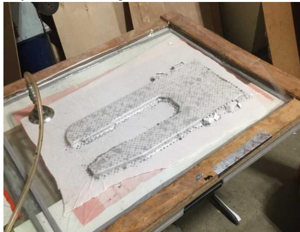
Figure 39. Drivetrain Plate being cured using a glass table.
