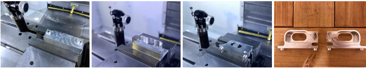
Figure 34: Dropout mount geometry after each machining operation final left and right dropout mounts.
