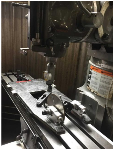
Figure 44. Sprocket being trammed in and preparing to drill the holes for the engine mount. Note that the probe feature here was not the one used. The proper probe that was used is the same test indicator found in Appendix E.
