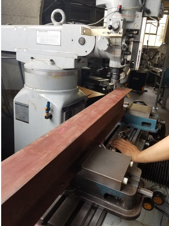
Figure 44. Shimming the I-beam
