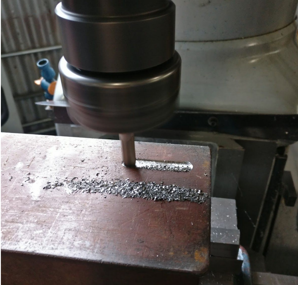
Figure 46. Machining slots into the I-beam
