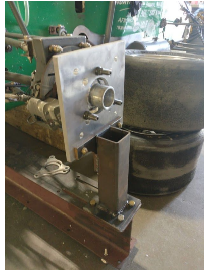
Figure 61. Jig in place for proper welding location (left), final rear support arms (right)
