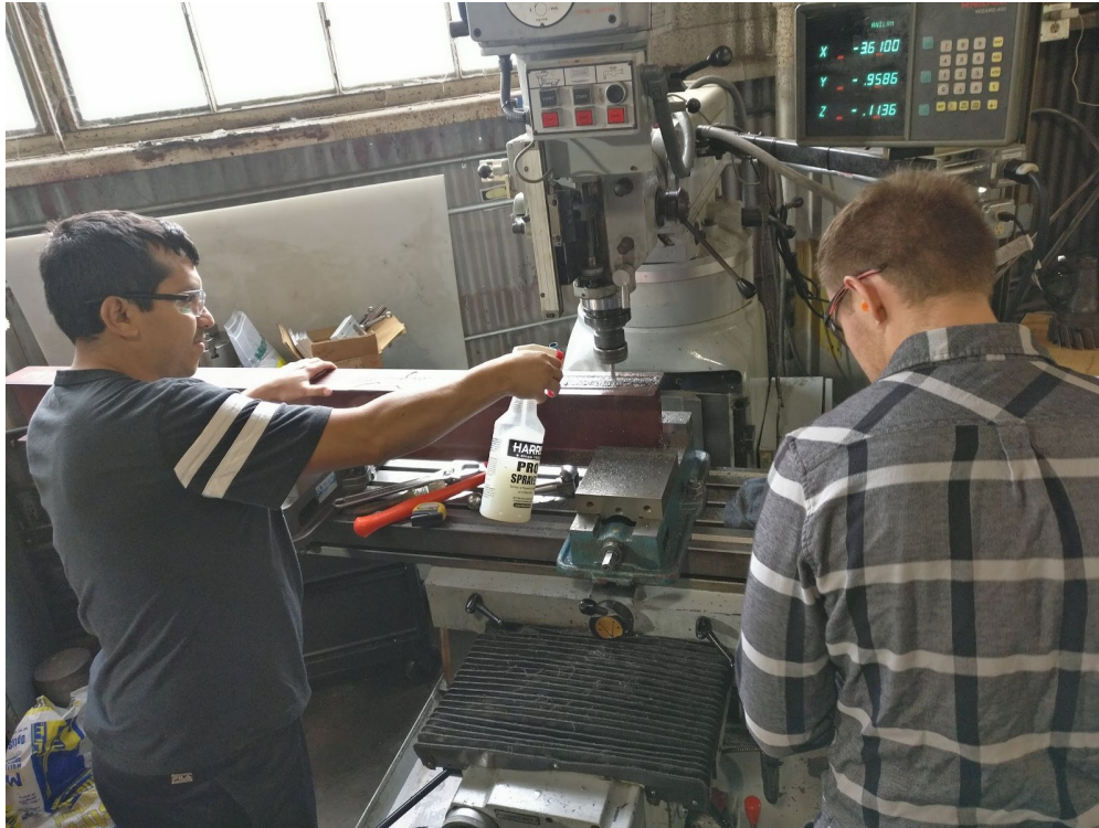
Figure 45. Working on machining the I-beams
