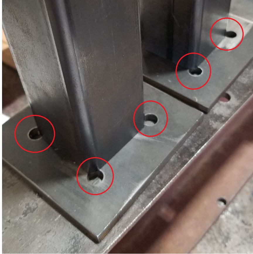
Figure 53. Incorrectly cut rear hub stand plates
