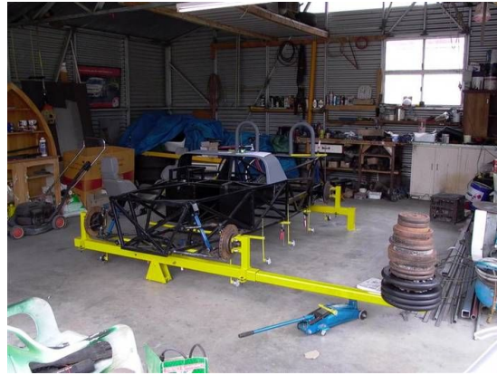
Figures 39 and 40. Dial indicators located on chassis to get deflection
