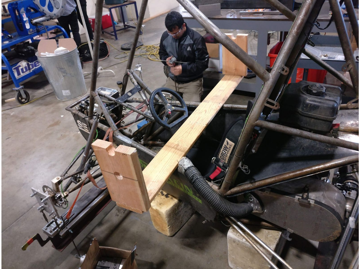
Figure 76. Wood bracing used to hold extra weights
