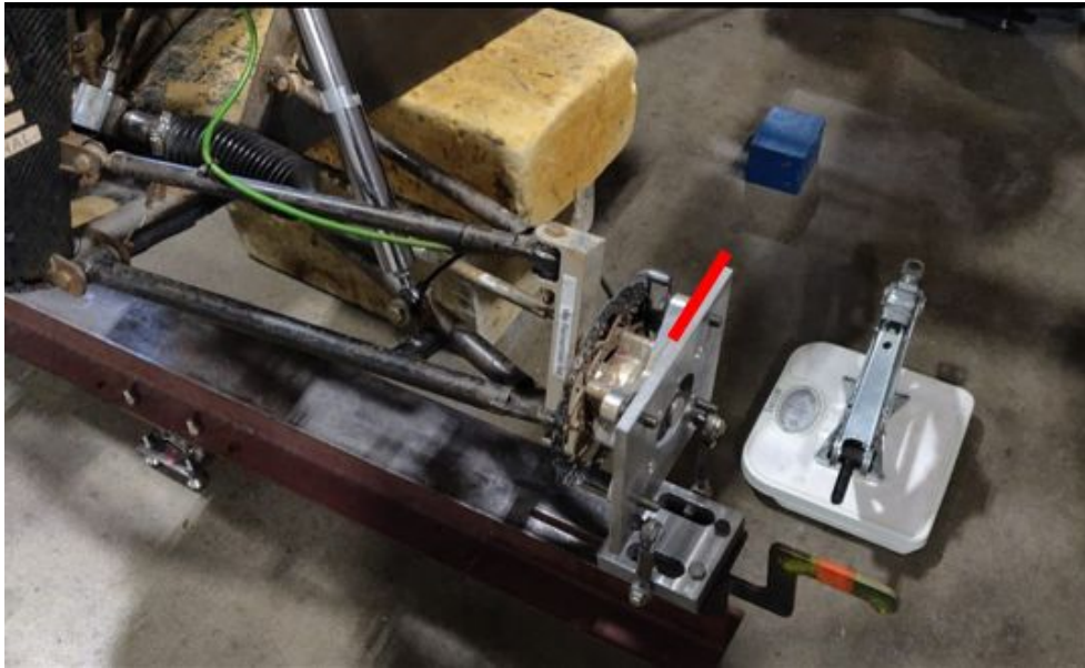
Figure 20. Shim stock applied for rear adjustments.
