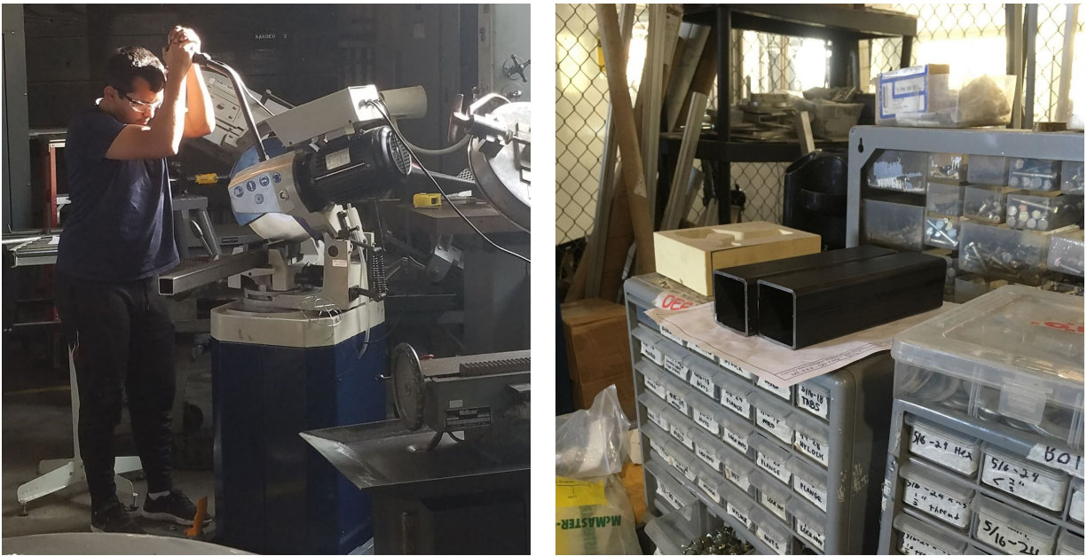
Figure 60. Omar cutting the square tube stock (left) and the final cut tubes (right)
