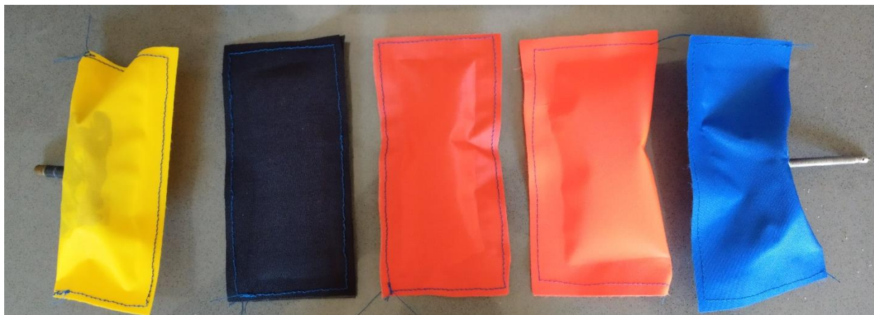
Figure 16: Sample Pockets for Proof Loading Verification
