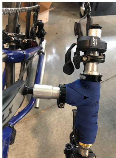
Figure 32. The gear shifting levers. Bottom is shift down, Top is shift up.
