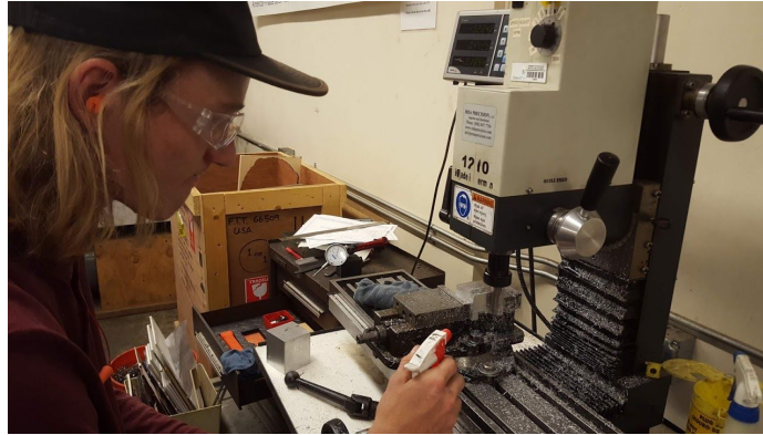
Figure 25. Manual milling operation for upper rotor mount.
