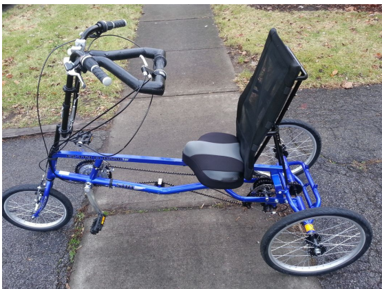
Figure 1. A MonoMano trike designed for one-handed steering, shifting, and braking.
