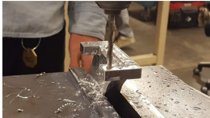
Figure 29. Drilling operation for caliper mount.
