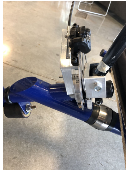
Figure P.5. Steering lock caliper & rotor assembly
