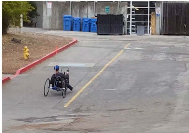
Figure 33. Testing functionality by riding up a 5% grade hill.
