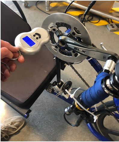
Figure 34. Load Input Steering Test
