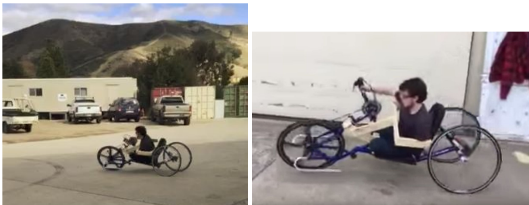
Figure 10. Alex testing the lean-assisted steering capabilities of the prototype.
