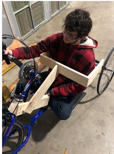
Figure 9. The concept prototype for lean-assisted steering.
