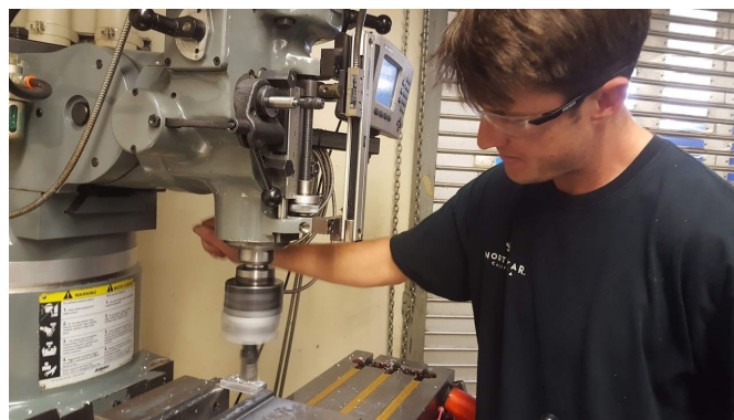
Figure 28. Boring operation for lower rotor mount.
