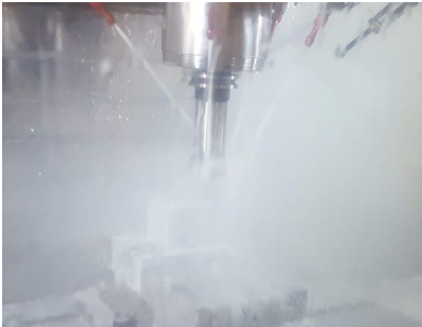
Figure 23. CNC milling operation for upper rotor mount
