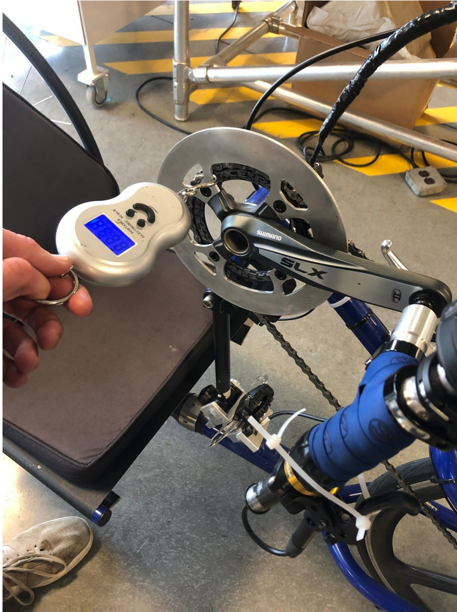
Figure I.4. Load Input Steering Test
