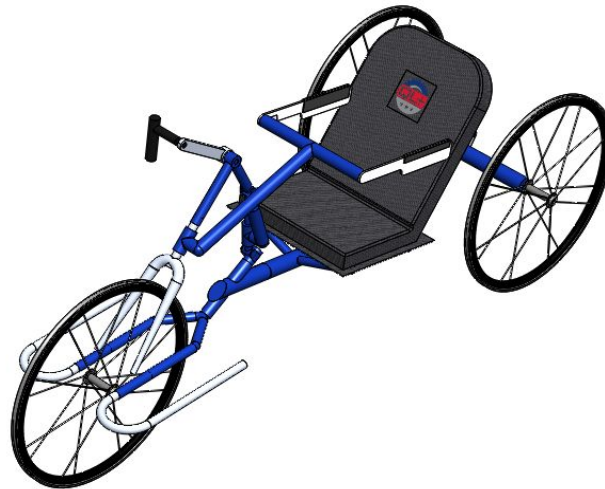
Figure 11. CAD model of the lean assisted steering prototype.
