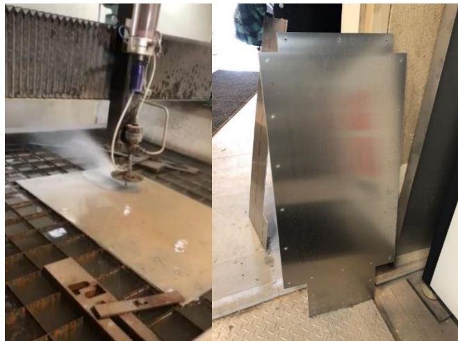
Figure 39. Waterjet cutting the sheet metal platform surface.
