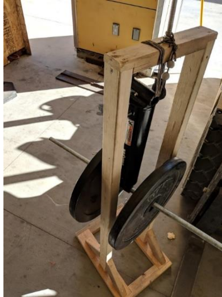
Figure 48. Hydraulic load test set-up.
