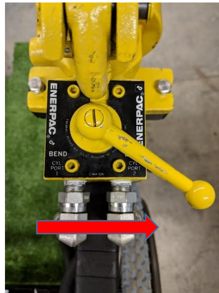
Pump switched to extension
