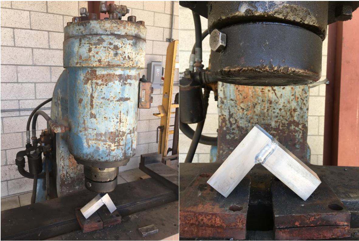
Figure 46. Sample weld test piece in hydraulic press.
