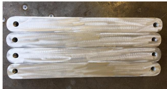
Figure 37. Linkage arms during paint preparation.
