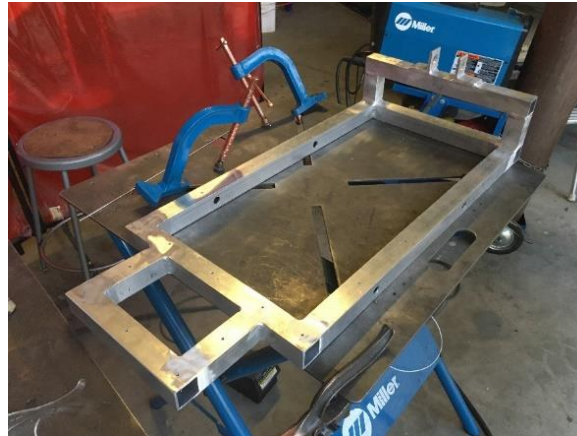
Figure 38. Fully welded platform tube frame.
