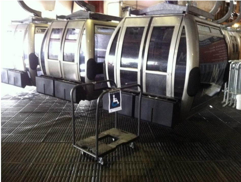
Figure 3. Modified utility cart currently in use. Picture courtesy of Josh Pighetti
