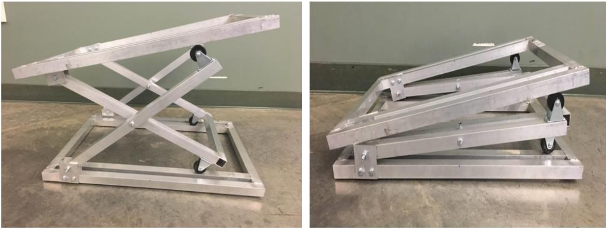
Figure 27. Structural Prototype in raised (left) and lowered (right) positions.
