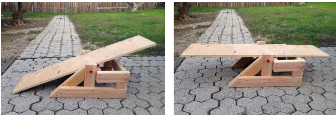
Figure 12. Concept prototype built to correct gondola height (10 inches), shown with the ramp down (left) for loading and up (right) for transportation and transferring into the gondola.
