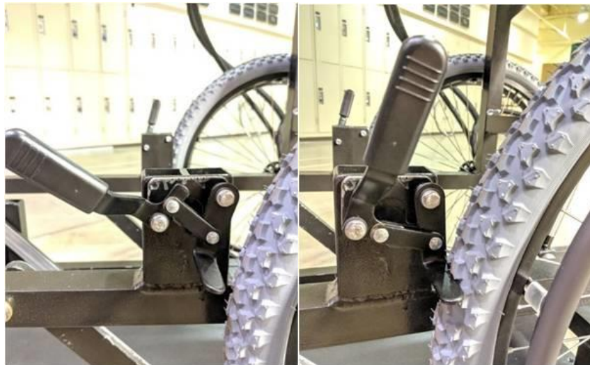
Figure 49. Wheel locks in open (left) and locked (right) positions.
