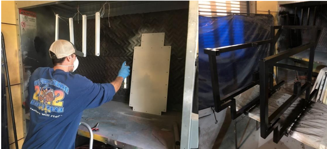
Figure 42. Painting all manufactured aluminum components with aluminum primer and paint.
