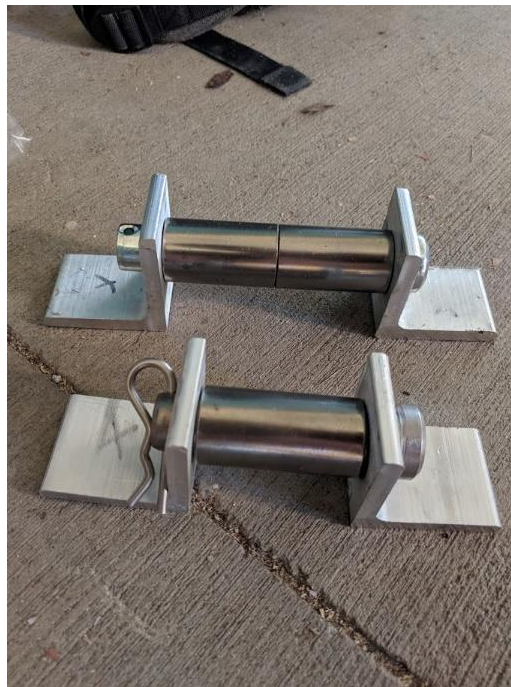
Figure 43. Hydraulic bracket assembly including clevis pins, cotter pins, and sleeve bearings.
