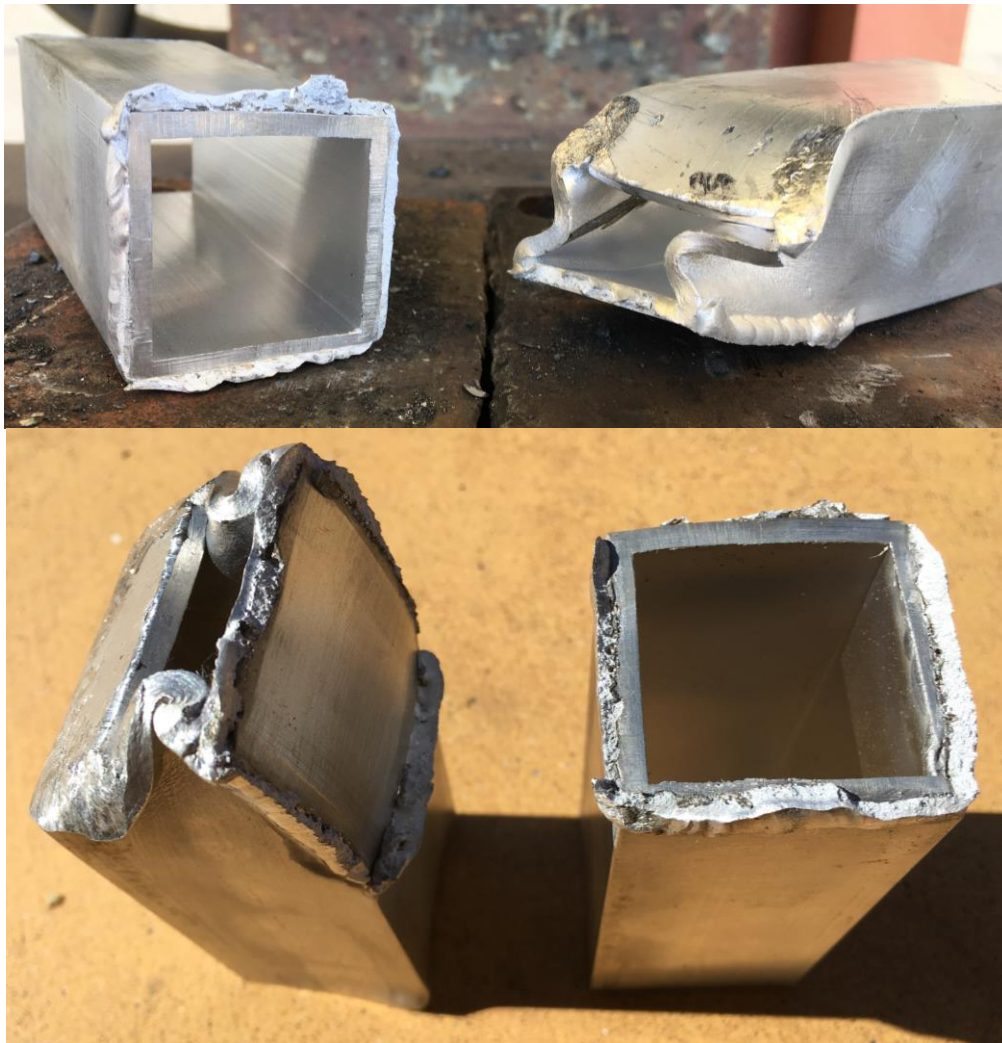
Figure 47. Weld break test pieces from 1 st (top) and 2 nd (bottom) rounds.
