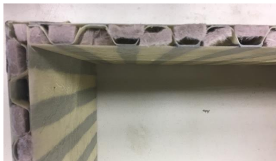
Figure 6.2. Corrugate wall installed with aerogel fiberglass composite.
