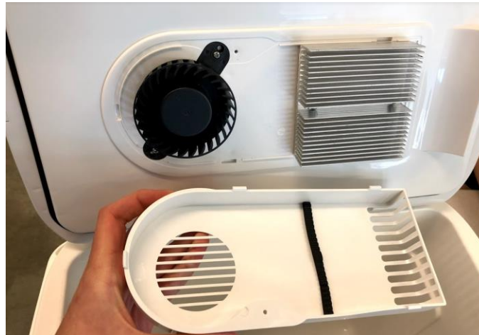
Figure 2.2. Cold side of Peltier setup in the igloo iceless.
