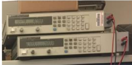
Figure 1. Picture of the power supply.
