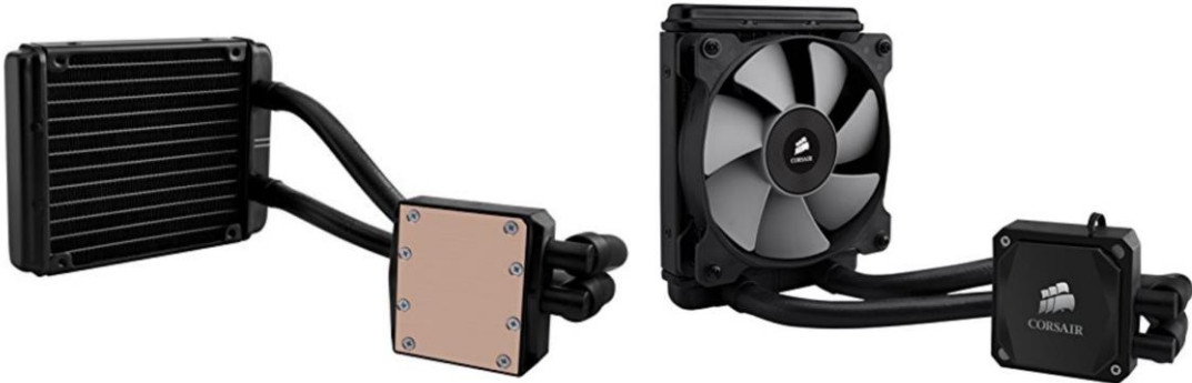
Figure 5.9 Front and back images of the Corsair series H60 CPU cooler. [16]
