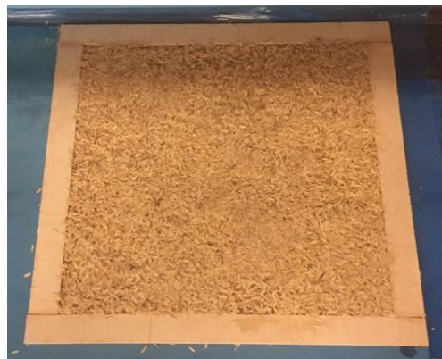
Figure 7.15. Manufactured test specimen using rice hulls and silicone caulking.
