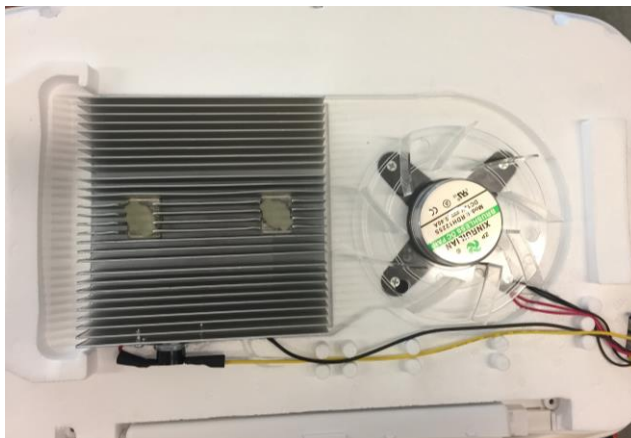
Figure 2.3. Hot side of Peltier setup in the Igloo Iceless Refrigerator.
