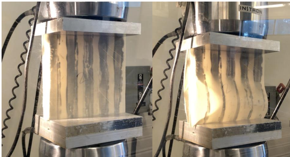
Figure 7.1. Corrugated panel under distributed vertical load, failure at 6000 lbs.
