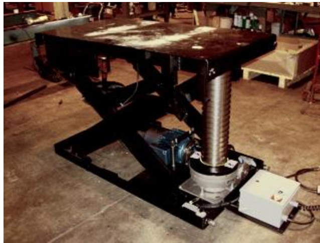
Figure 2.2. Model 24-SL-020 motor driven spiral lift table with vertical adjustment when the helical column is rotated to change the table's height.
