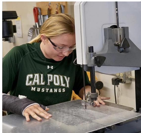
Figure 6.6. Cutting the panels for the belt housing.
