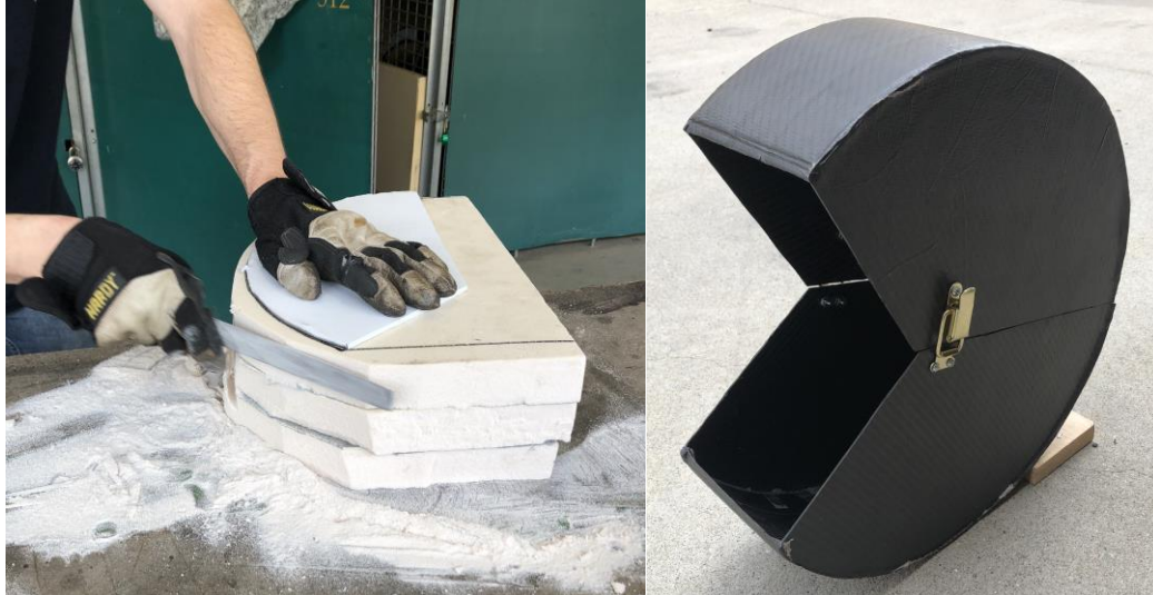
Figure 6.2. The carbon fiber mold being prepared and the finished housing
