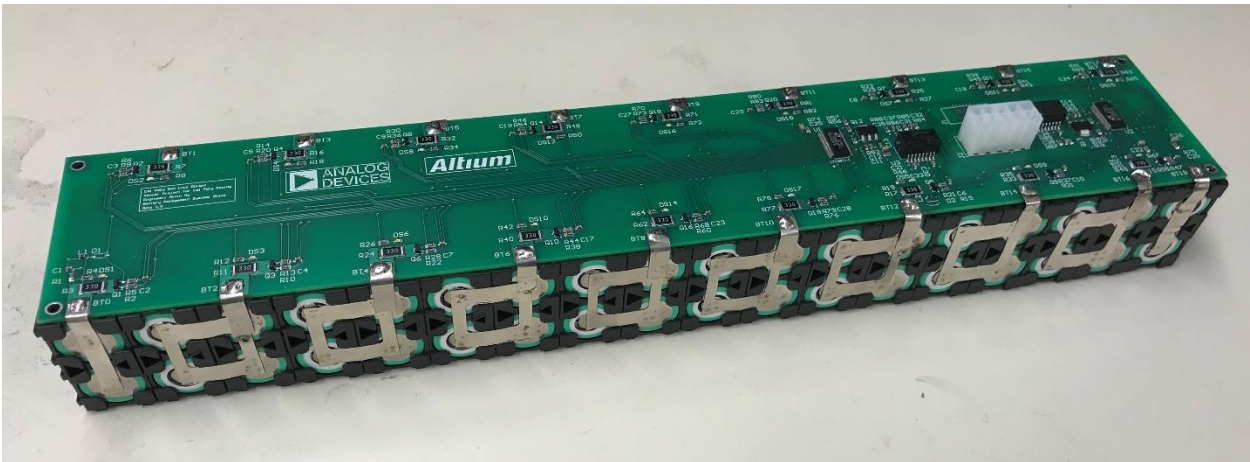
Figure 41: BMS Slave Test Module
