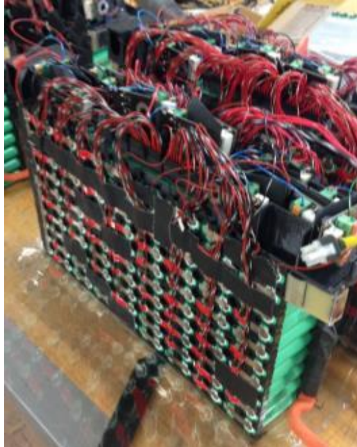
Figure 2: Current BMS Module Integration
