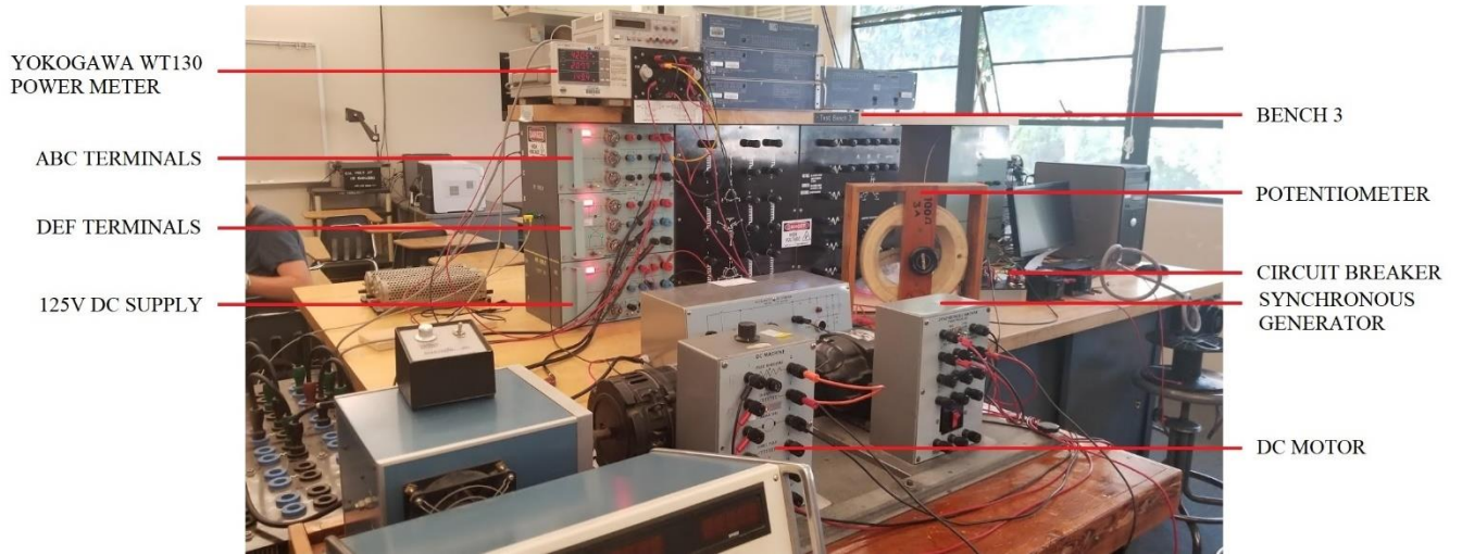
Figure 10. Islanded Mode Testbench Setup
