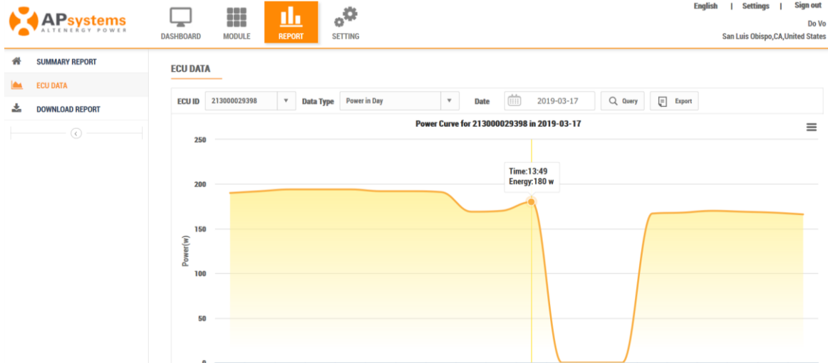
Figure 43. Output Power of the Microinverter using EMA
