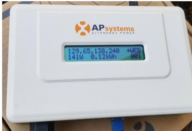
Figure 12. Microinverter's Output Power Display on the ECU
