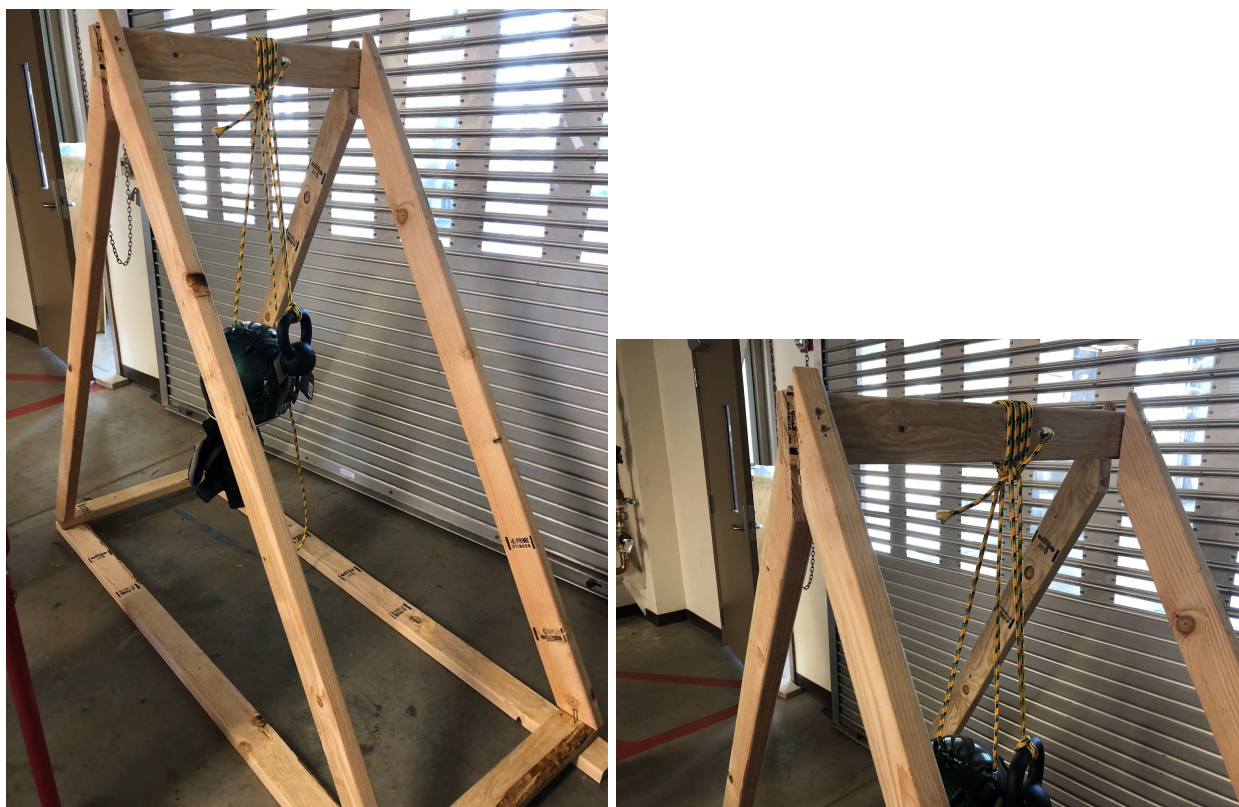
Figure 7: Construction of the impact tester is shown.
