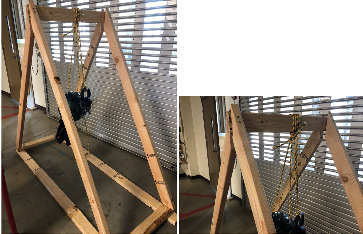
Figure 8: Construction of impact tester is shown.
