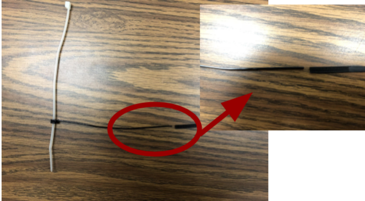
Figure 11: The failure of the zip tie attachment is shown, as encountered on the first trial dropping from 60 degrees with the 17.5 lb weight.
