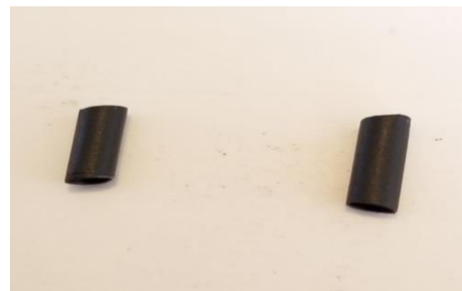
Heat shrink cut down to 10mm each.
