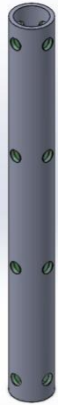
Figure 4.2.1: Rendering of the design freeze for the temperature-sensing section of the probe body. The rest of the body includes non-modified tubing to house the wiring and connect to the circuit board.
