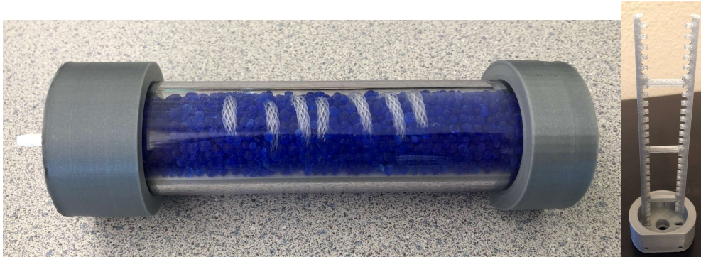
Figure 6: From left to right: final dehumidification chamber and 3D-printed support piece attached to one of the two 3D-printed caps
