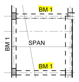
\*ALL B1 BEAMS BEAR ON MASONRY SHEAR WALLS
