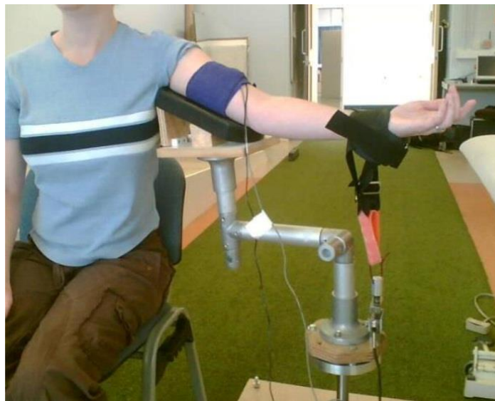
Figure 3: Force production vs. EMG signal intensity test setup [4]
