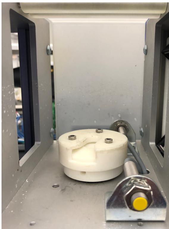
**Figure 3.7** – A view of the syringe chuck inside the SpinCAM.
