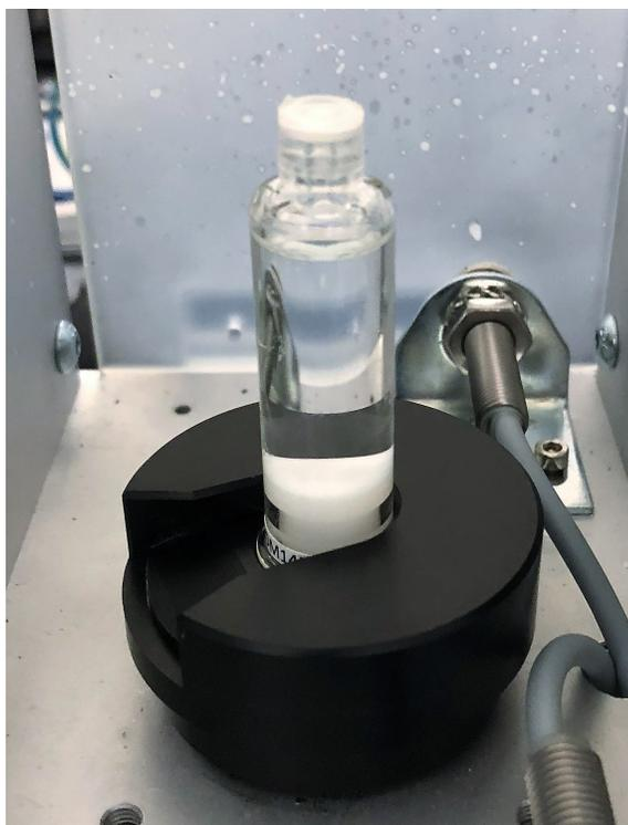
**Figure 3.6** – 5 mL cartridge placed on the chuck inside the SpinCAM.
