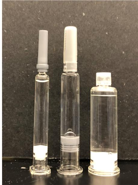
**Figure 3.8** – A front view of the 1 mL syringe, 2.25 mL syringe, and 5 mL cartridge
