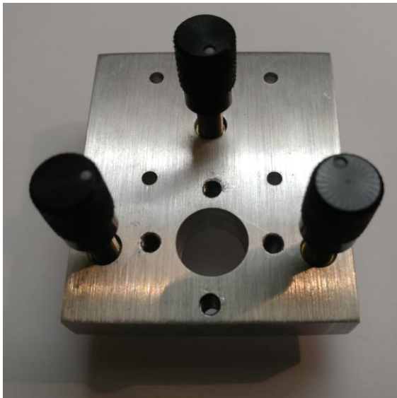
Figure 3: Device top plate with fine adjustment screws and embedded bushings (top view)
