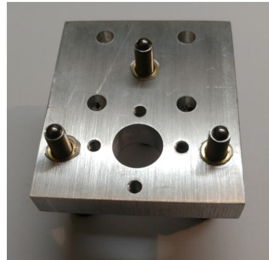
Figure 4: Device top plate with fine adjustment screws and embedded bushings (bottom view)
