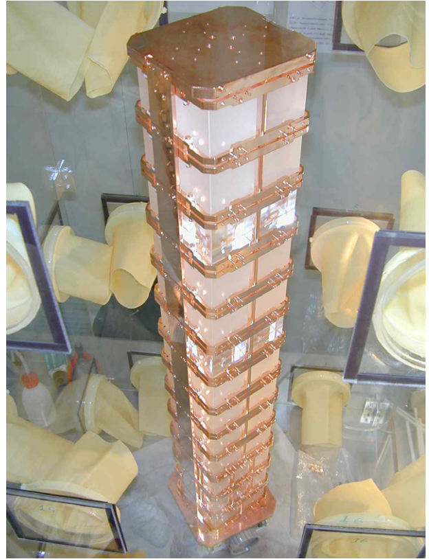
Figure 1. The CUORICINO tower inside a nitrogen-fluxed glove-box, during the final assembly of the detector.
