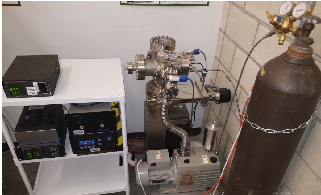
Figure 3.5: Experiment electrical equipment, vacuum chamber, rotary pump, and propellant feed system.
