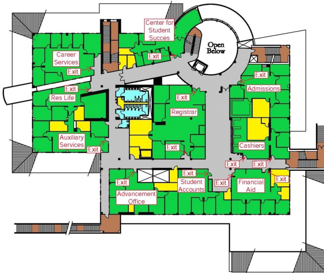
Figure 4-5 - Second Floor Occupancy Exits
