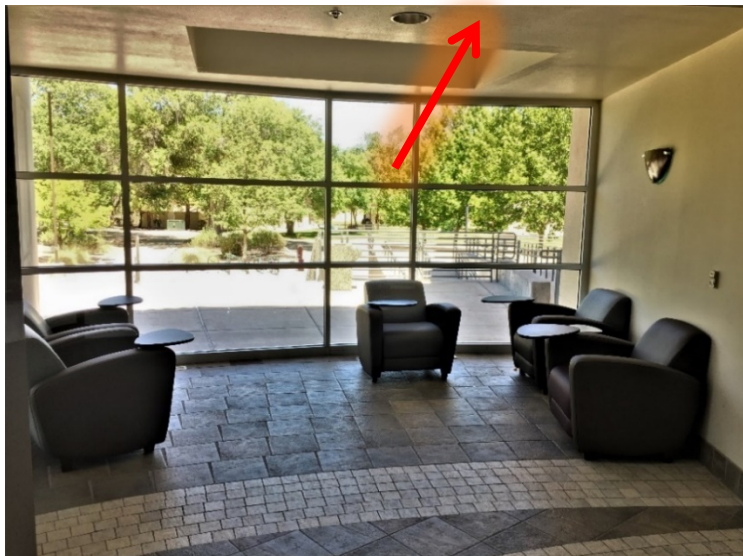
Figure 7-6 - Recommended Secondary Smoke Detector Placement
