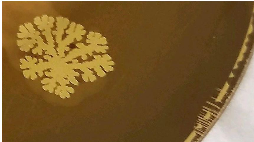
Figure 4.1 Sputtering Adhesion: HMDs primer adhesion issues during spin-coating, often indicated by the floral-like pattern
