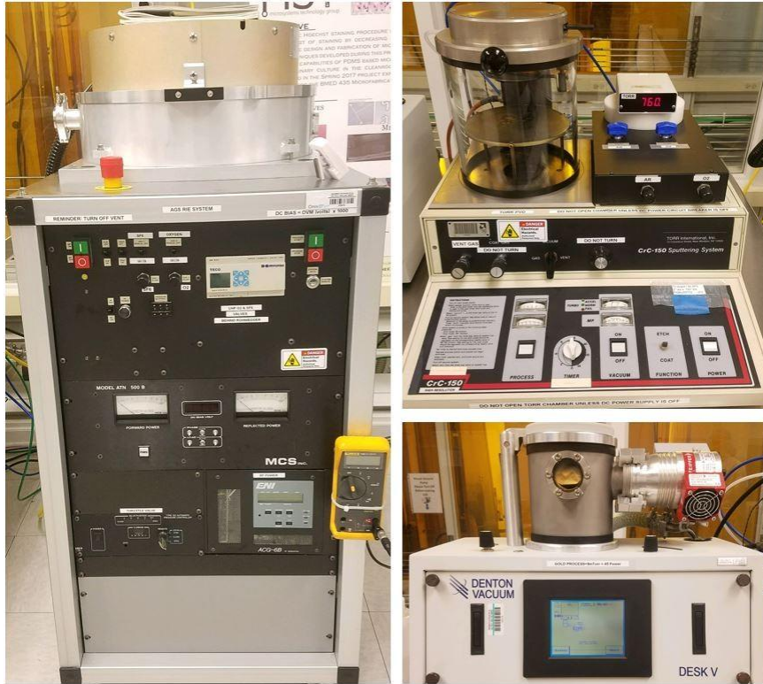
Figure 3.15 Machines for Physical Vapor Deposition: Left: Reactive Ion Etch machine. Top Right: Chrome sputter machine. Bottom Right: Gold sputter machine.
