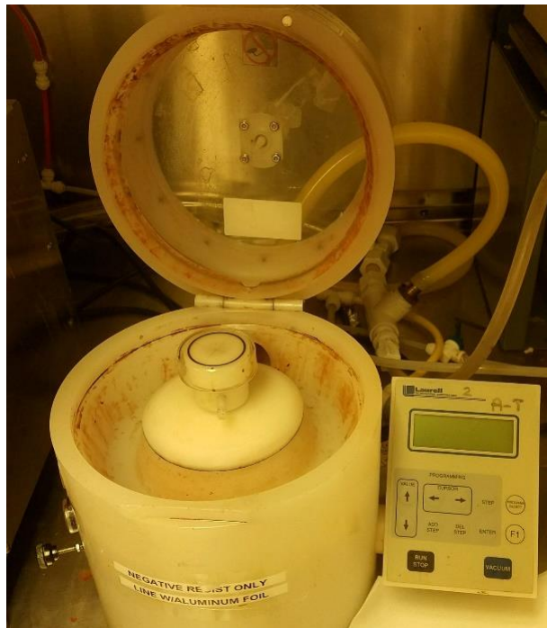
Figure 3.7 Photoresist Spin Coater: Spin coat machine used to spin-on various layers of photoresist
