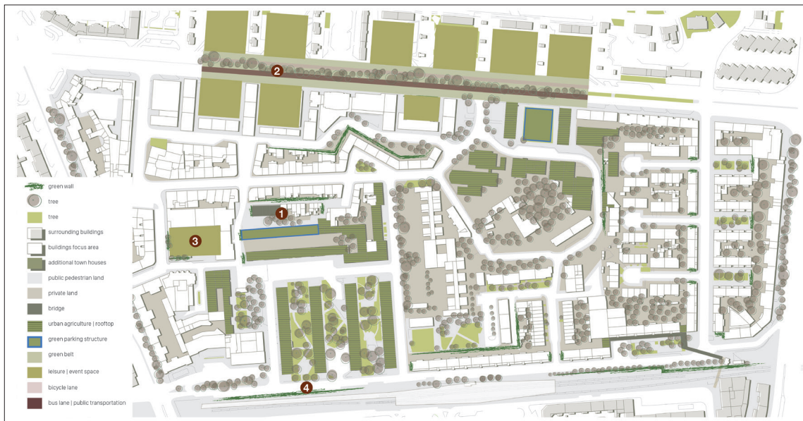
Figures 3 a, b & c: The site plan and two details from the proposal by Hannah Tesch, Kyle Ferguson, and Nishita Kandikuppa. Detail 1 shows a new structure with a community garden on top of an existing surface parking lot. Detail 3 shows the concept to revitalize an existing abandoned plaza.
