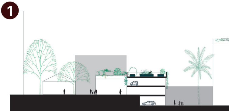
Figures 3 a, b & c: The site plan and two details from the proposal by Hannah Tesch, Kyle Ferguson, and Nishita Kandikuppa. Detail 1 shows a new structure with a community garden on top of an existing surface parking lot. Detail 3 shows the concept to revitalize an existing abandoned plaza.
