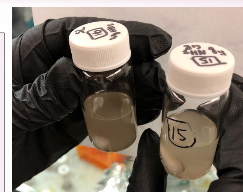
Figure 4. Vials of two samples of nanodiamonds undergoing liquid amination.
