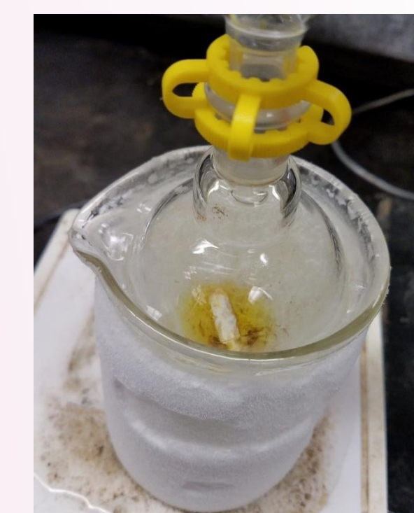
Figure 6. NH 3 condensing in reaction flask containing NDs and stir bar.
