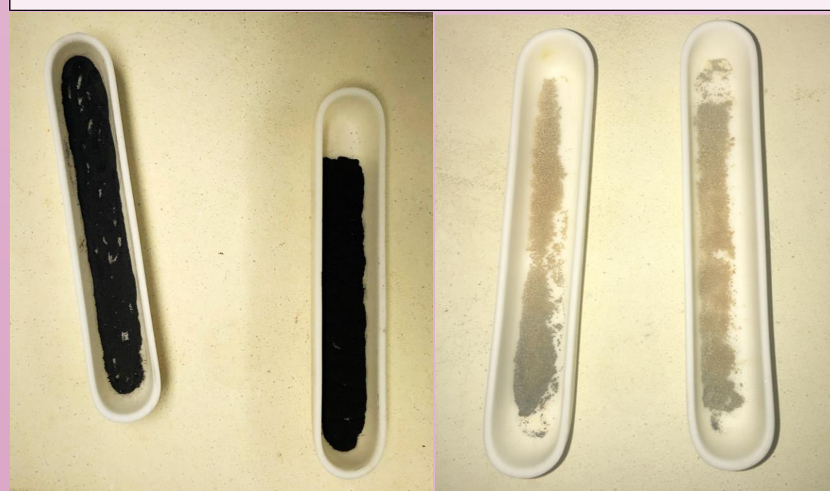
Figure 2-3. HPHT nanodiamonds in boats prior to oxidation (left) and after nearly 24 hours of oxidation at 550°C (right). A light tan color is sign of well-oxidized nanodiamonds.
