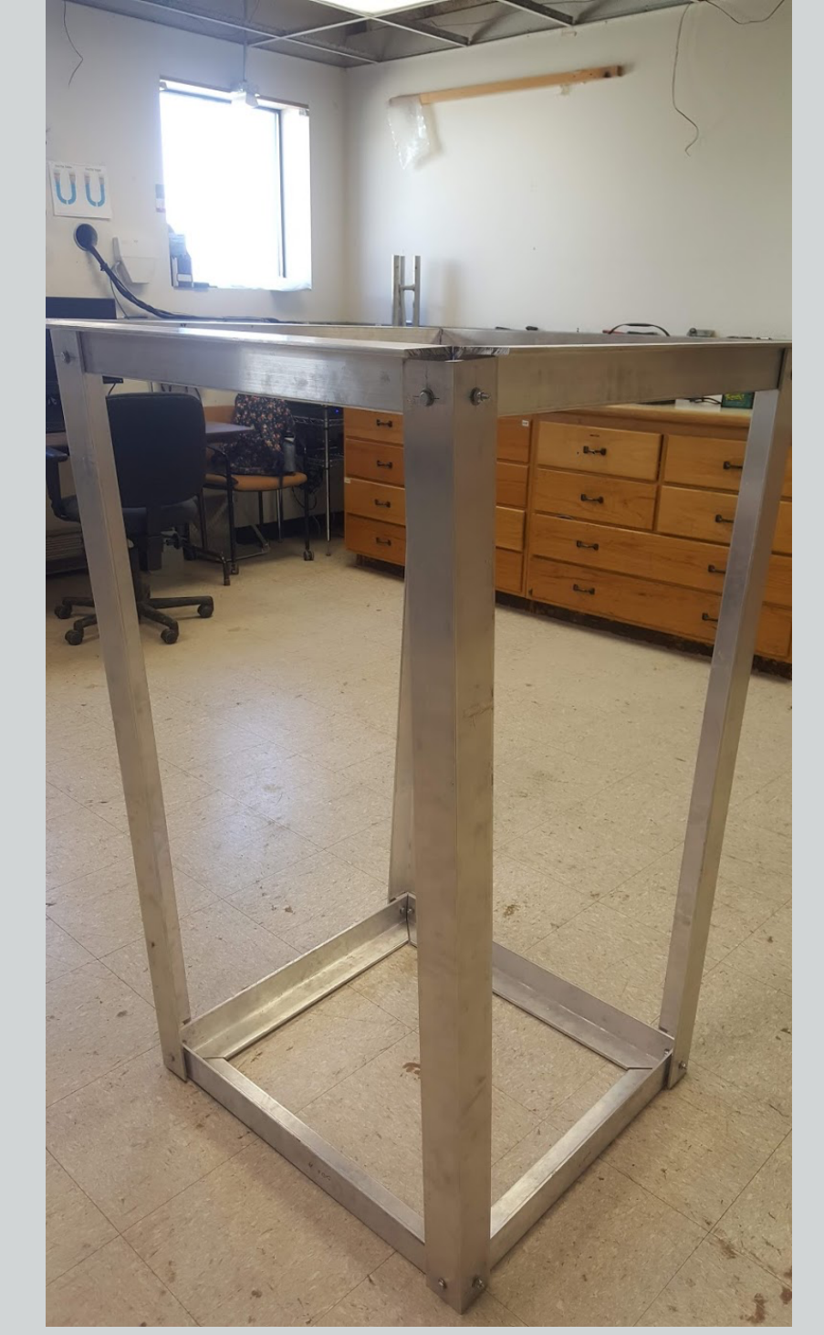
Figure 5: Each midpoint was bolted with a quarter inch bolt using a socket wrench
