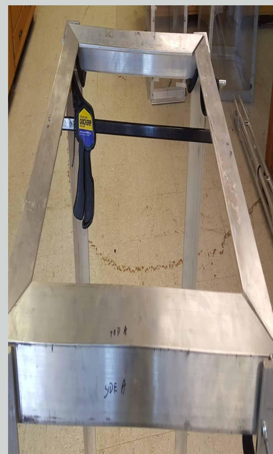
Figure 6: Top view of the snow machine that depicts the 45 degree angle cuts
