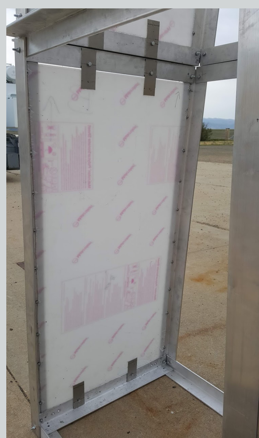
Figure 7: Plexiglas used to make the sides of the snow machine
