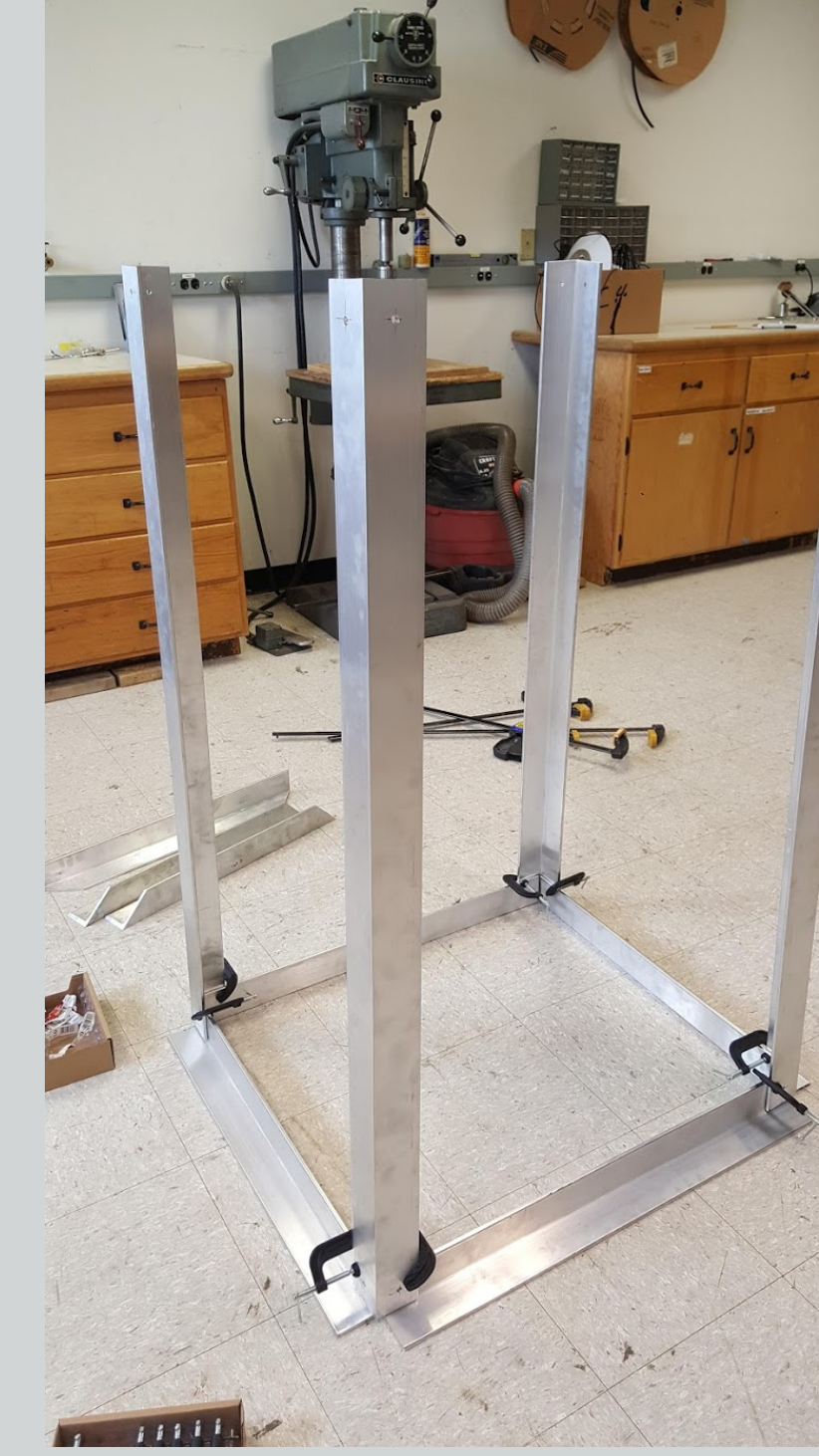
Figure 3: The standing model of the snow machine before being bolted together
