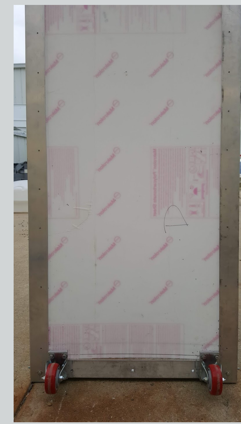
Figure 9: Wheels on the bottom are used for easier transport of the system by tipping the system onto the wheels and moving it around and the holes drilled between them will be used for bolting a support plate for the Plexiglas to stay intact
