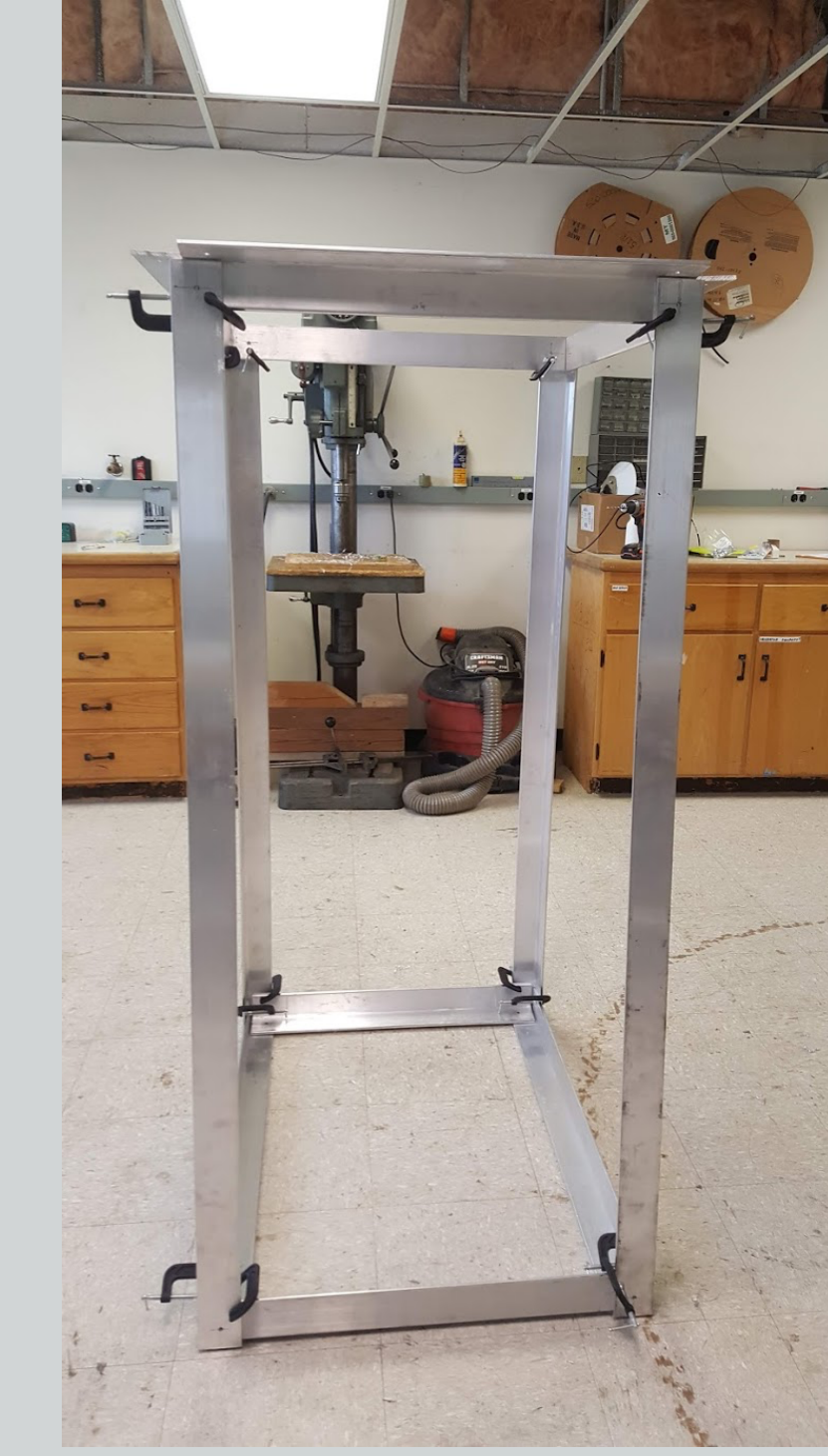
Figure 4: Completed standing model, where each clamp represents the point at which each strut will be bolted
