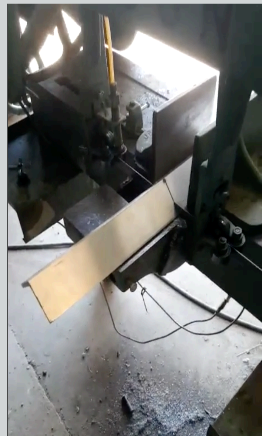
Figure 1: This is a horizontal band saw used to cut the aluminum struts
