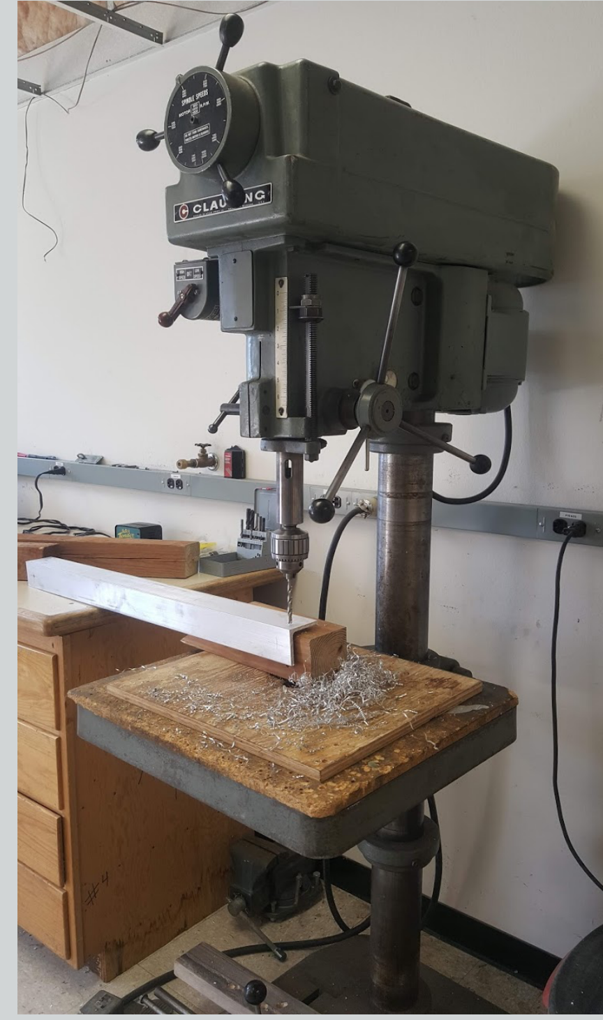
Figure 2: Drill press used to make holes on the marked midpoints of the struts
