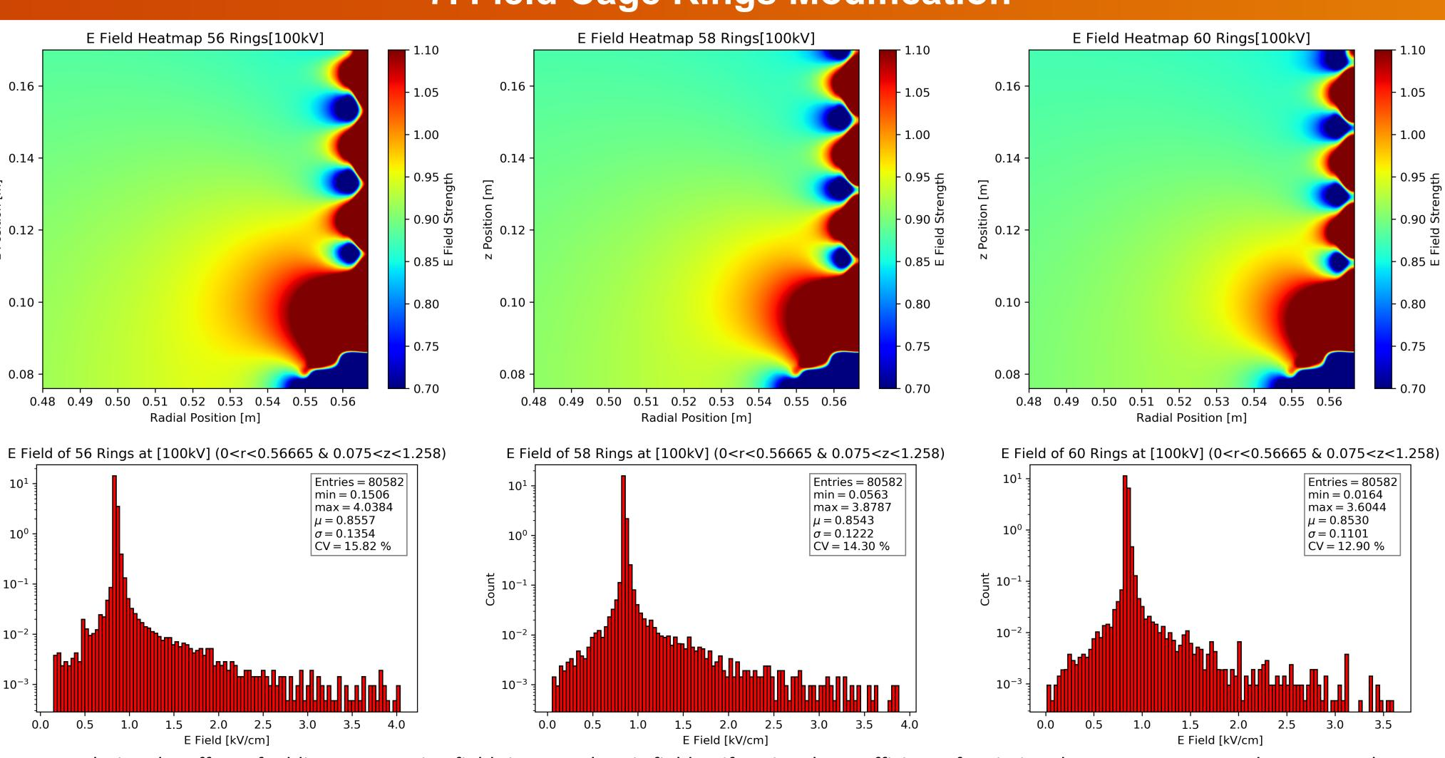
By analyzing the effect of adding or removing field rings on electric field uniformity, the coefficient of variation decreases as expected. However, the high number of rings would limit the efficiency of light collection by the UV-sensitive silicon photomultipliers (SiPMs) arrange right behind the field shaping copper rings. .
