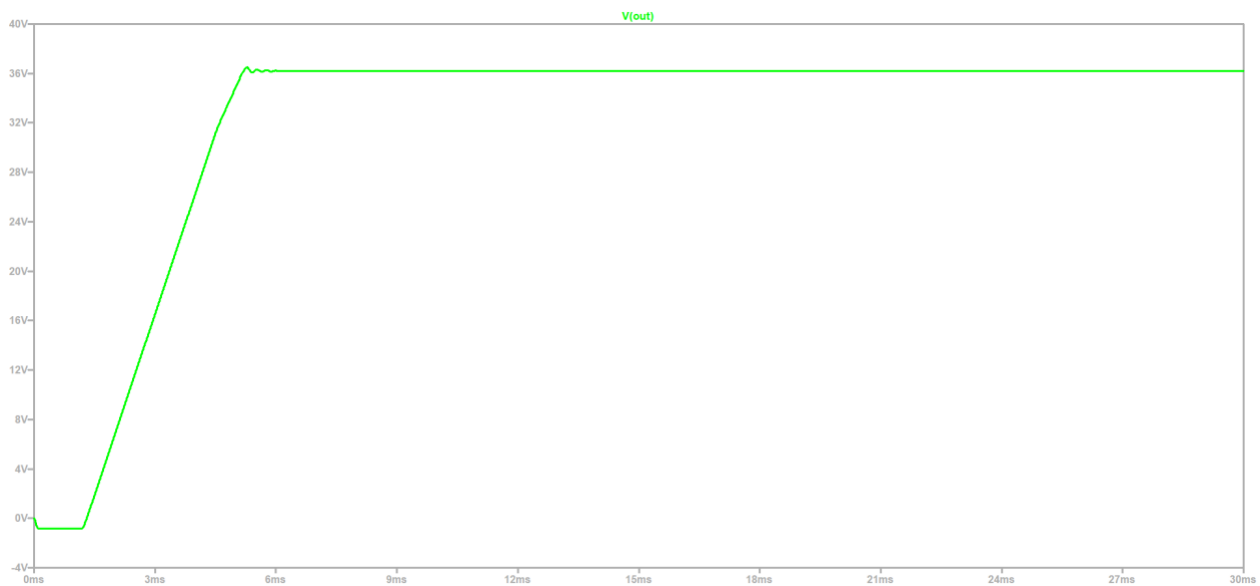
Figure XVIII: 36.19 V output voltage and less than 1 V output voltage ripple with 3.7 An electronic load.
