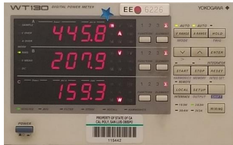
Figure 15. Power, Current, and Voltage Measurements from the Yokogawa Power Meter
