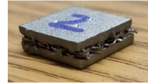
Figure 66: Control test specimen 2 was fully crushed during compression testing.
