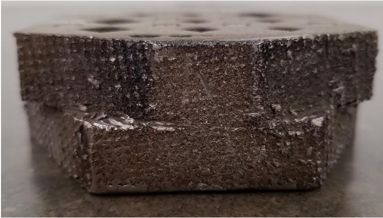
Figure 71: Removal of the support structure from the base of the hexagon leaves behind a surface too tough for any profilometry measurements.
