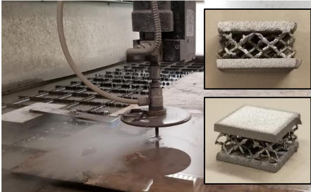
Figure 63: Plywood with a water-jet cut stencil to support the disk samples was used.
