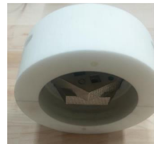
Figure 72: Enclosures were developed by Empowering Technologies for the peening of these specimens.
