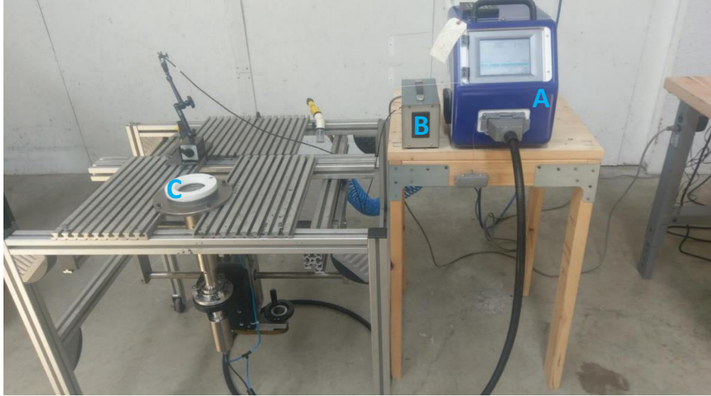
Figure 73: USP treatment set-up at Empowering Technologies with A: StressVoyager Central Unit, B: Ultrasonic Generator, and C: Enclosure Base.
