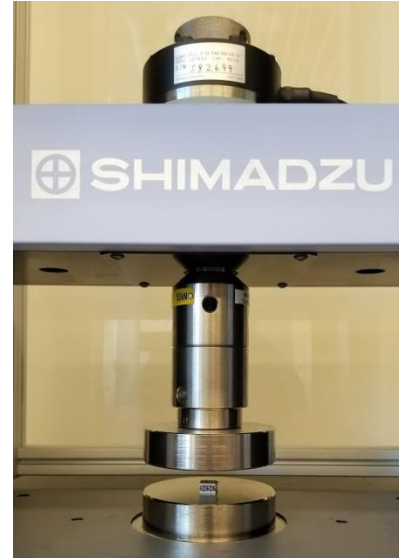
Figure 64: Shimadzu compression test was set-up as such for these tests.
