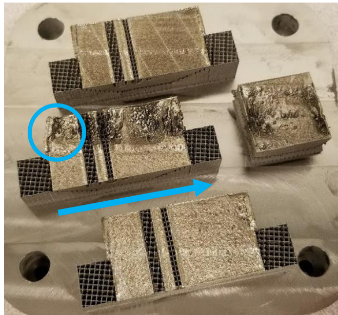
Figure 39: Recoater arm impacted the curled-up area indicated by the circle. Recoater movement direction is indicated by the arrow. There is incomplete fill past the curled-up edge due to the inability of the recoater arm to push powder into this region of the build area.
