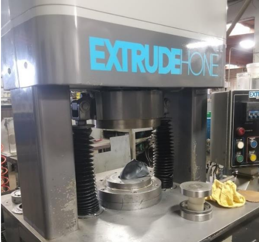
Figure 32: A two-way Extrude Hone AFM machine at the Extrude Hone facility in Paramount, CA. Note the abrasive media resting on the base plate.
