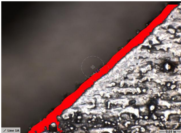
Figure 54: The red area denotes parasitic powder particles and surface material that was removed from this particular passage during AFM processing.
