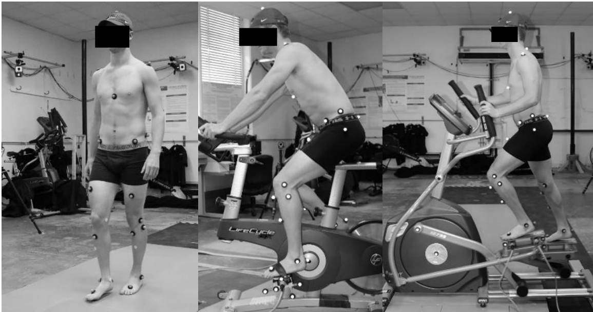
Figure 2.3: (Left) A participant walking along the walkway during a gait experiment, with the right foot contacting 1 of 3 ground force plates with motion analysis cameras recording G (two cameras are visible to the left and right of the participant's head in left photo). (Middle) pedaling the stationary bike instrumented with load cells on each pedal with markers tracking the pedal orientation. (Right) pedaling the elliptical instrumented with load cells on each pedal.
