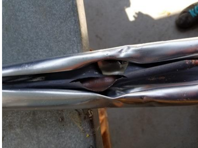
Figure 4.6: Ruptured Copper Heat Pipe and Aluminum Heat Transfer Fin
