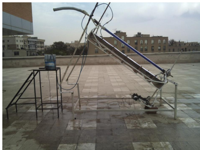
Figure 2.25: Experimental Setup for Sharif University Desalination System [25]
