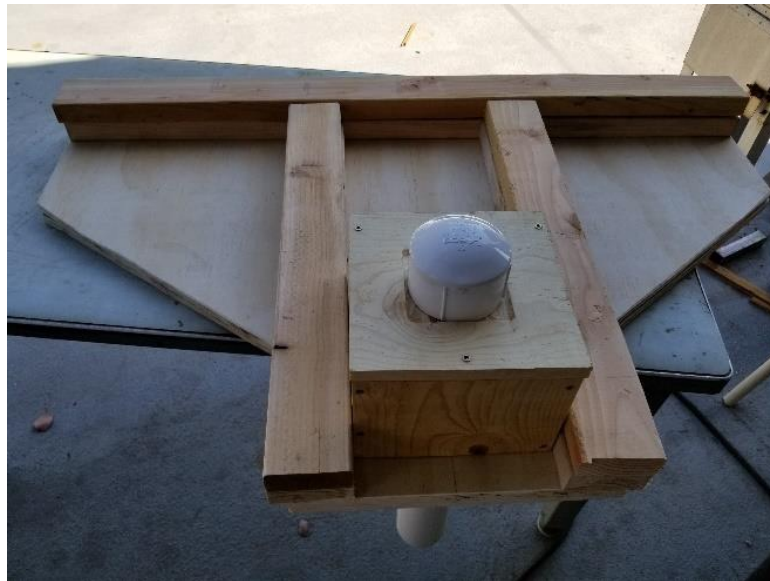
Figure 3.34: Bottom Endcap Gearbox and Evacuated Tube Holder
