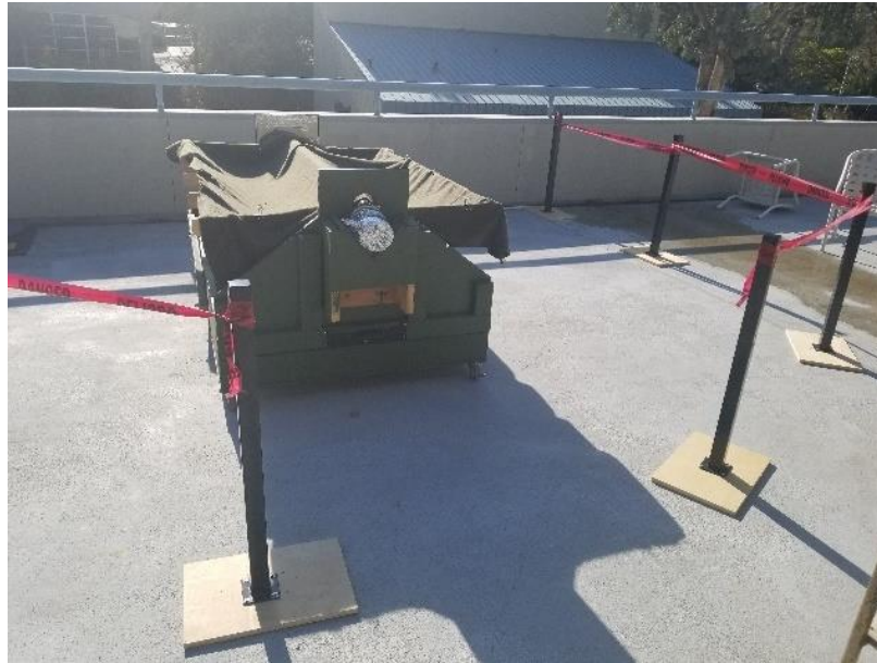
Figure 3.60: SODESAL System with Safety Barrier and Fire Blanket
