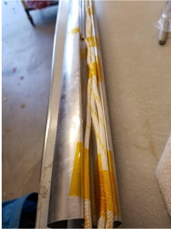
Figure 5.1: Aluminum Heat Transfer Fin and Thermocouples
