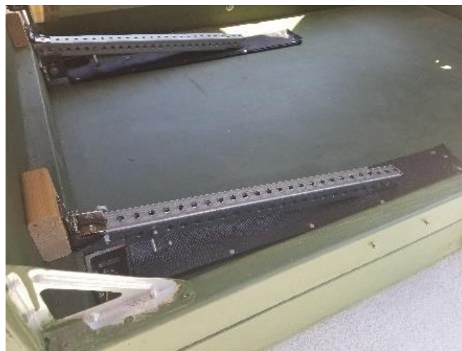
Figure 3.52: Protective Padding for Collapsed Supports
