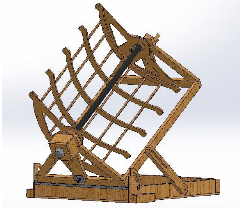
Figure 3.45: Fully extended and rotated SODESAL tracking
