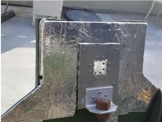
Figure 3.57: Bottom Endcap with Reflective Tape Figure 3.58: Top Endcap with Reflective Tape
