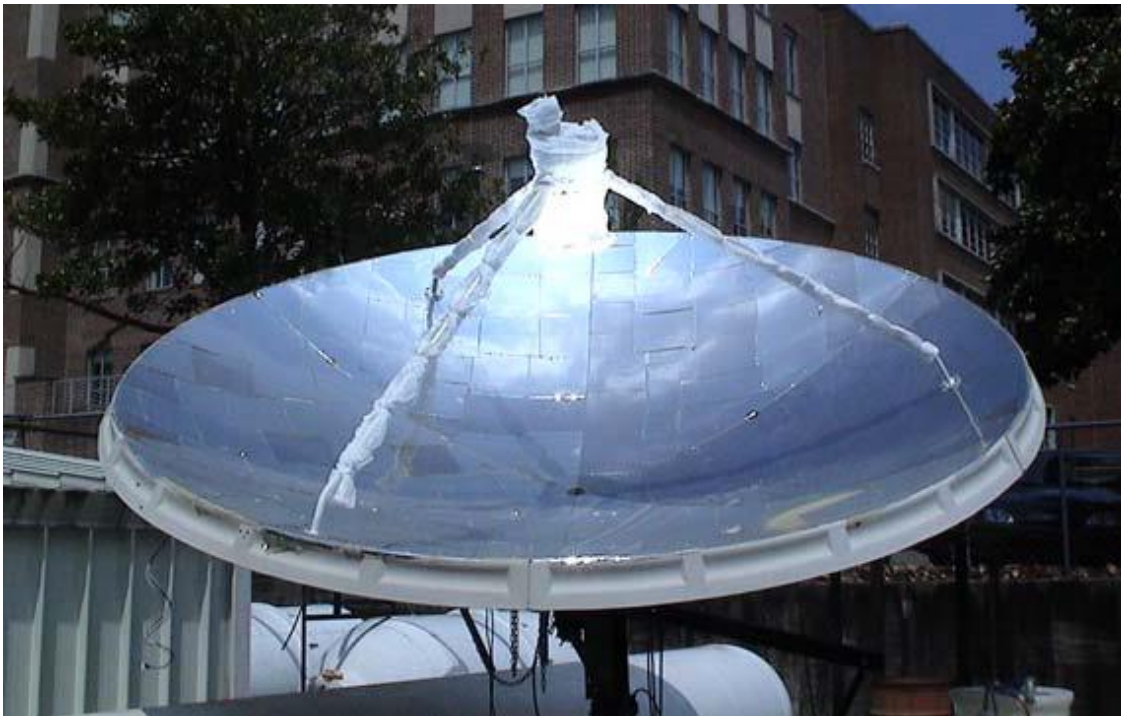
Figure 2.24: SESEC Parabolic Dish in Operation [24].
