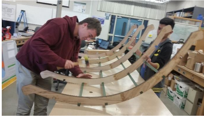
Figure 3.19: Mirror Rib Assembly with Support Rods
