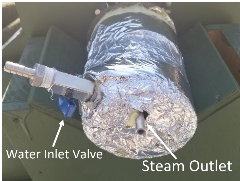
Figure 3.50: Mounted Boiler Wrapped in Insulation
