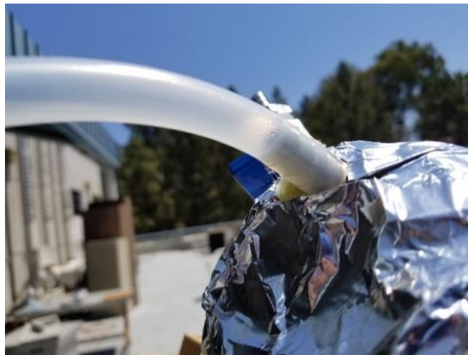
Figure 4.5: Steam Condensation Collection
