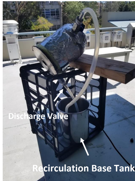
Figure 3.51: Recirculation Tank and Boiler Pump Test
