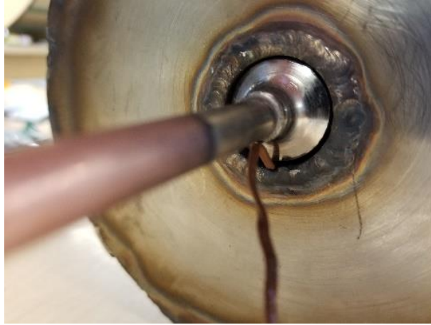
Figure 4.4: Boiler Thermocouple Position
