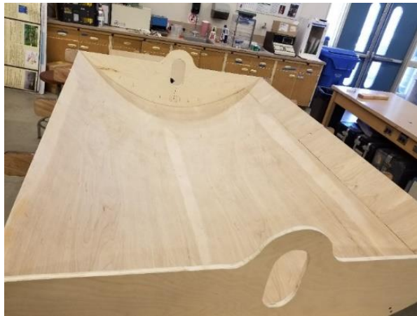
Figure 3.22: Parabolic Mirror with Wood Utility Panel
