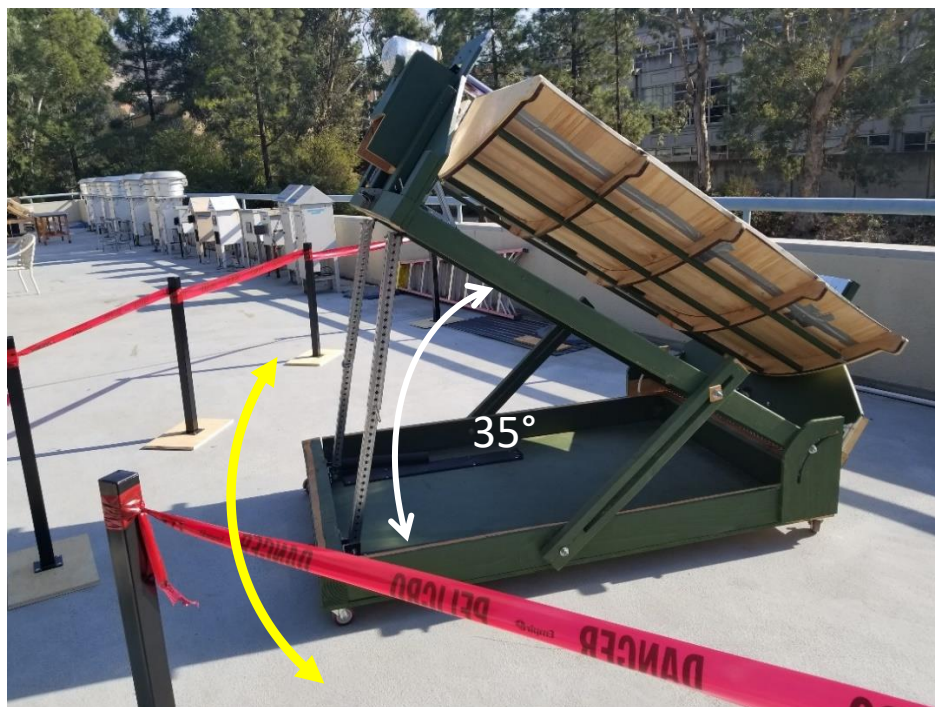
Figure 4.1: Phase 1 Experimental Design - mirror slope (white), sun tracking rotation (yellow)
