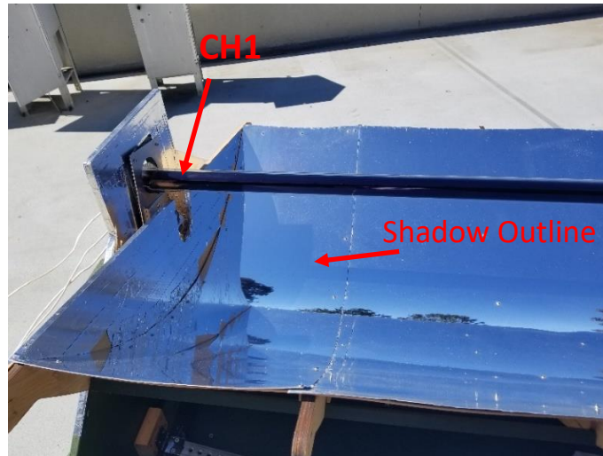
Figure 5.9: CH1 Shading by System Frame before Solar Noon.
