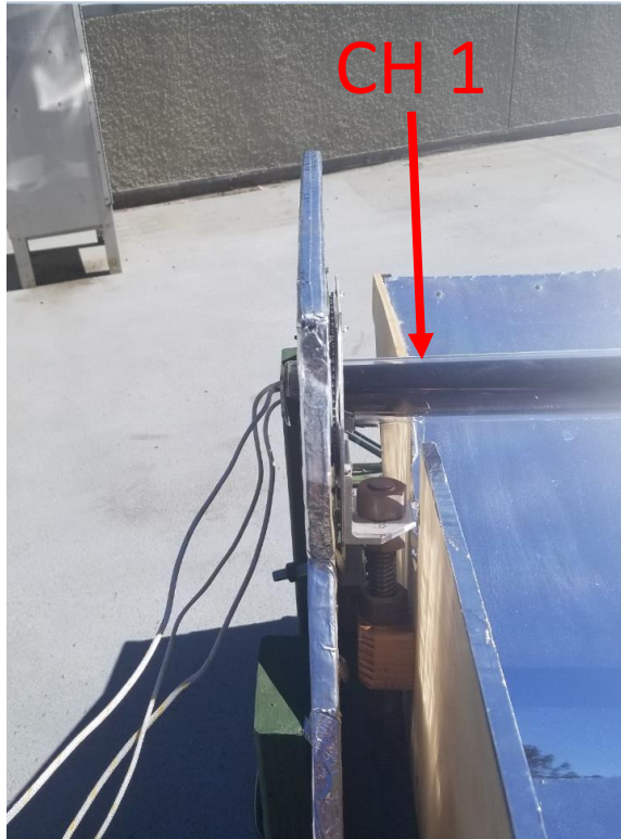
Figure 5.4: Evacuated Tube Extension & CH1 Location
