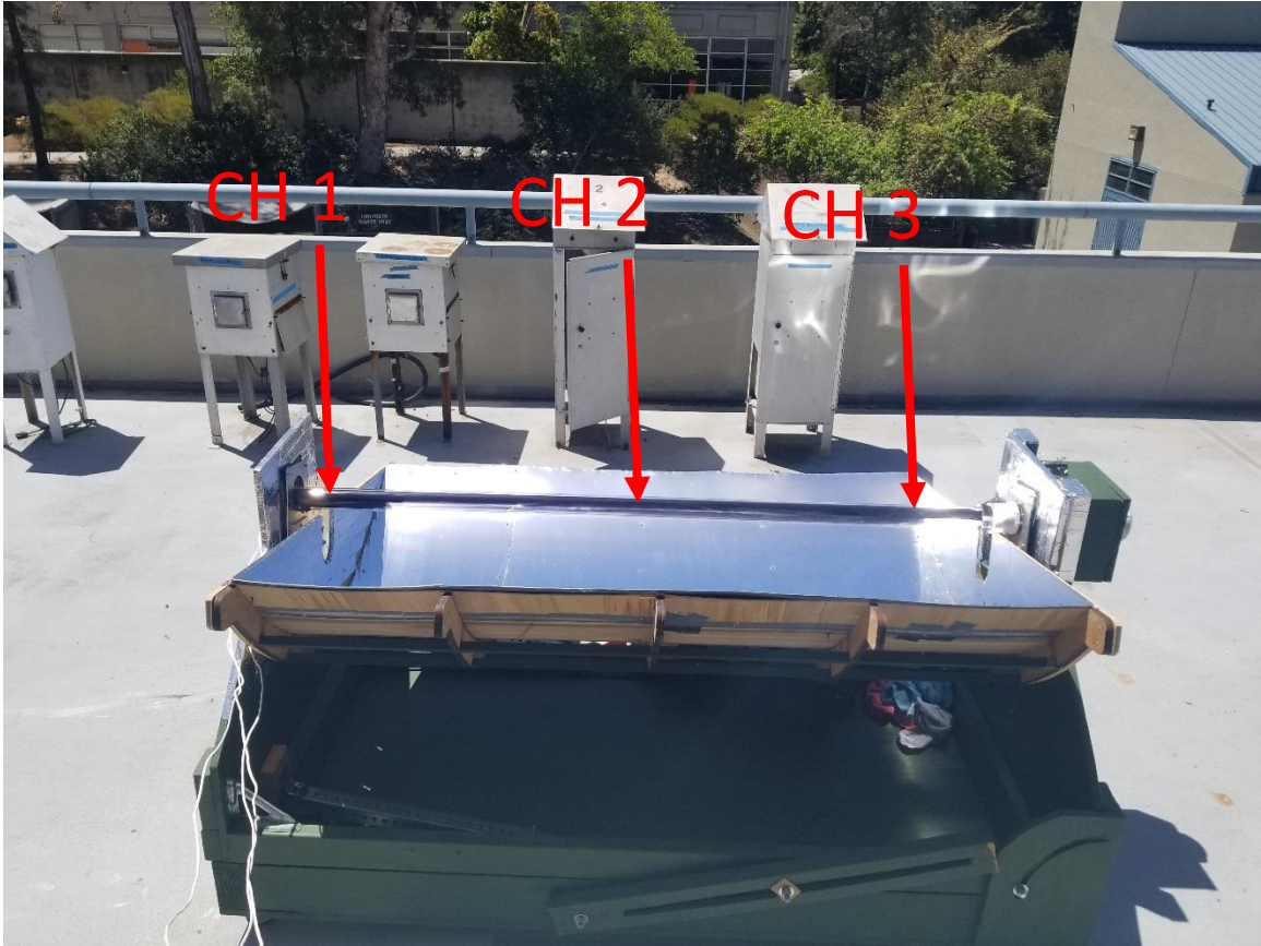
Figure 5.3: Thermocouple Locations for Lateral Heat Distribution Collection
