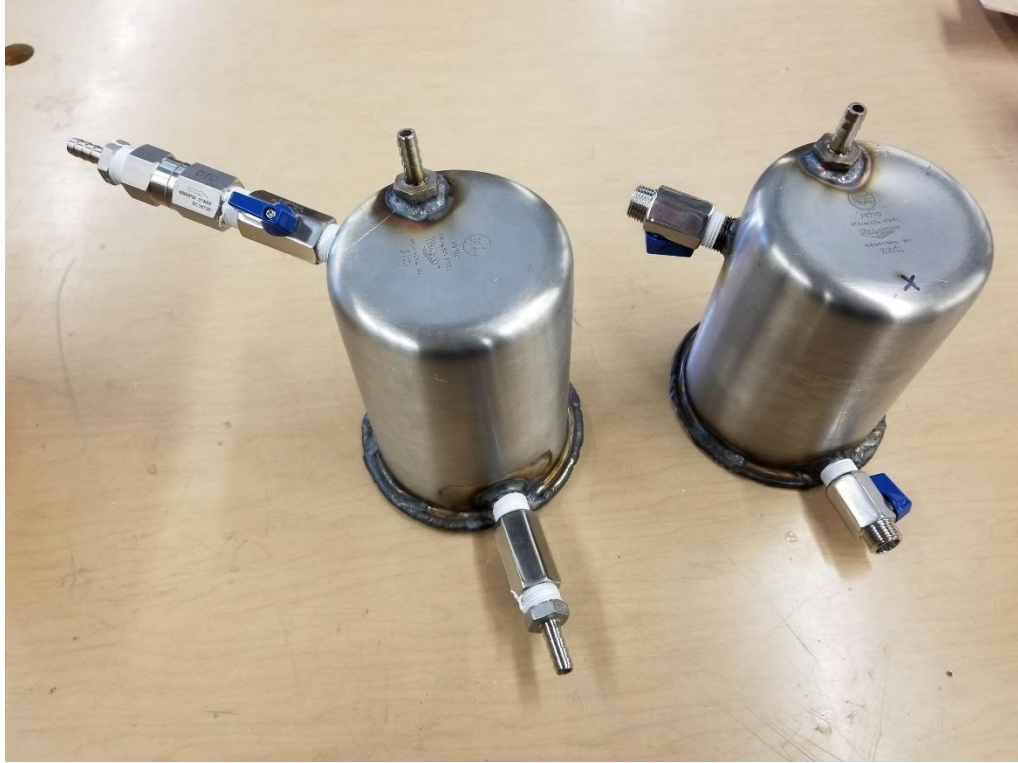
Figure 3.49: Finished Stainless Steel Boilers with Inlet and Outlet Valves
