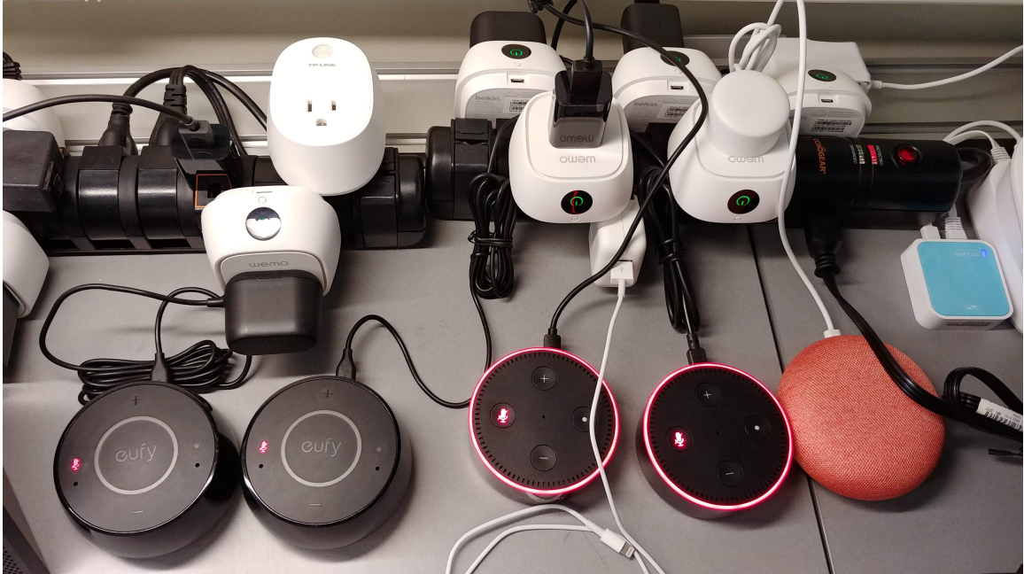
Figure 3.2: Smart Speakers Connected to Wemo Insight Switches
