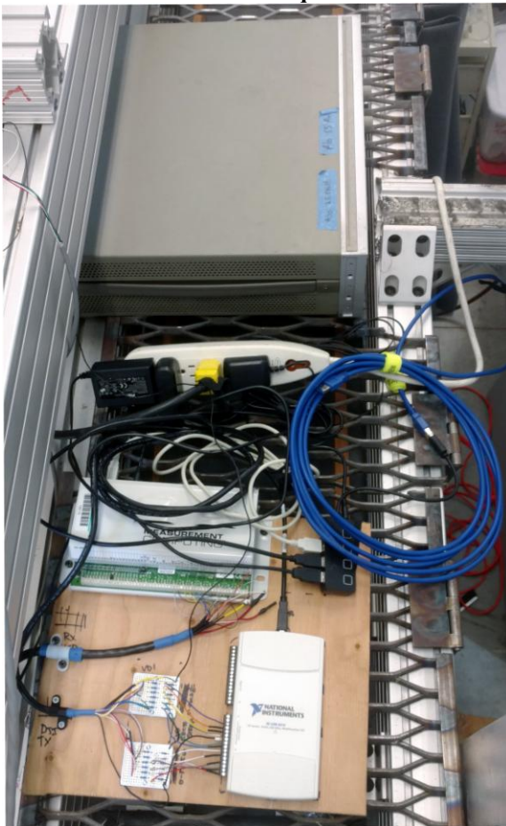
Tunnel Installation - Data Acquisition Hardware Pallet and Power Supply
