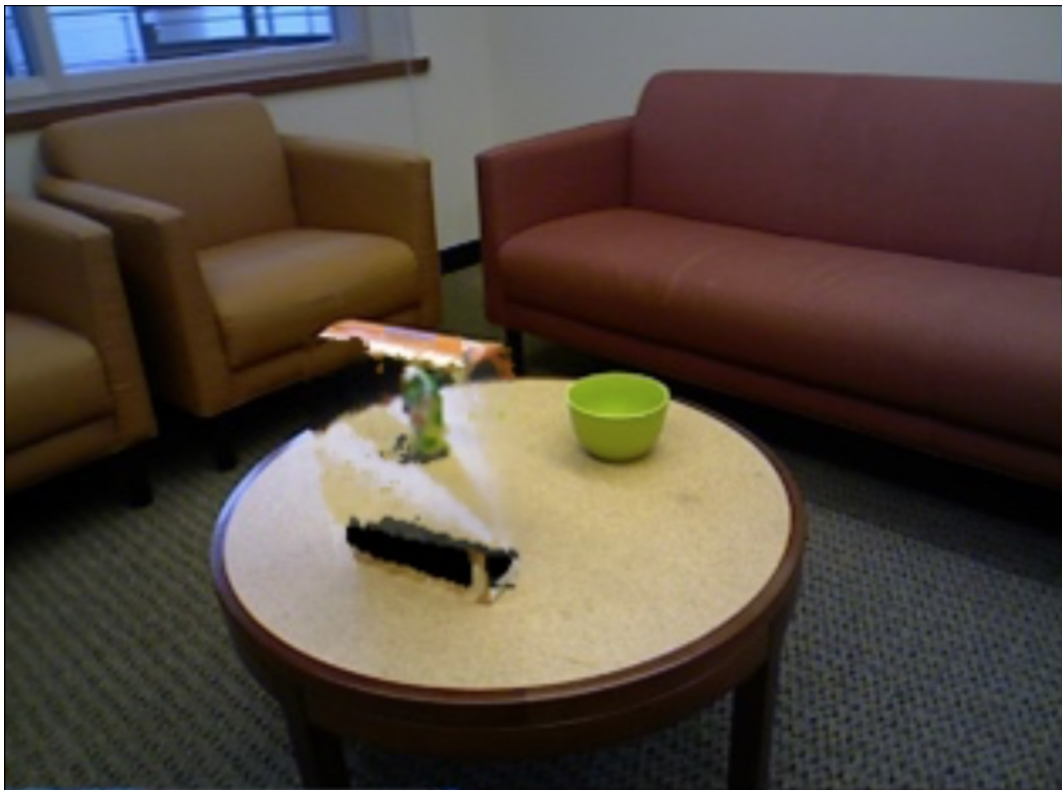
Figure 5.3: Result of removing a cereal box from the diminished reality method proposed by Nakajima et al [38].
