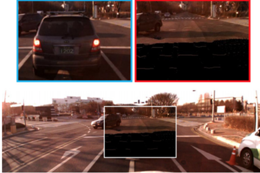
Figure 2.6: Seeing through a car using multiple cameras [43]. Top left image is from the back car’s perspective. Top right image is from the front car’s perspective.
