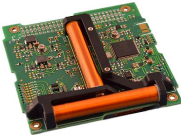
Figure 1.1: 3U CubeSat ISIS Magnetorquer Board.[1]
