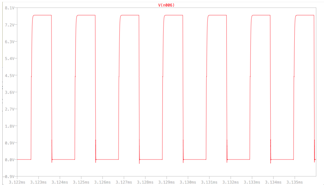
Figure 4-4 Duty Cycle of 47% at 48V input and 40V output
