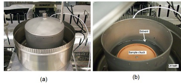
FIG. 2. Photographs of a conventional solvent annealing tool in this study; (a) overview; (b) the inside of the solvent annealing tool. The solvent temperature is controlled by an oil bath.
