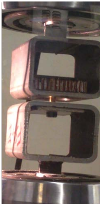
Figure 32. Pullout Test Setup
