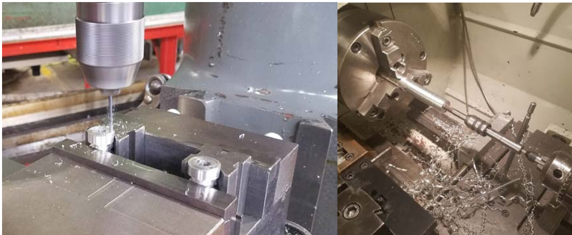
Figure 26. Potted Insert Manufacturing
