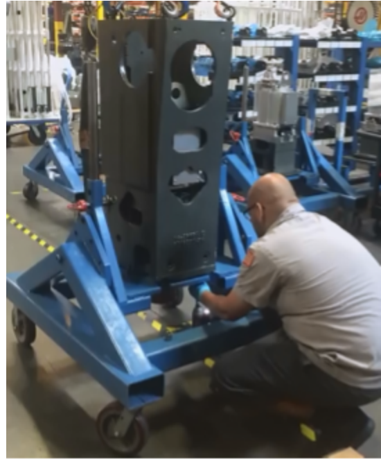
Figure 5. Securing the casting
