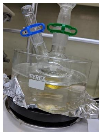
Figure 7.6. The sulfur shelling precursor ready for alternating injection to generate the ZnS shells.
