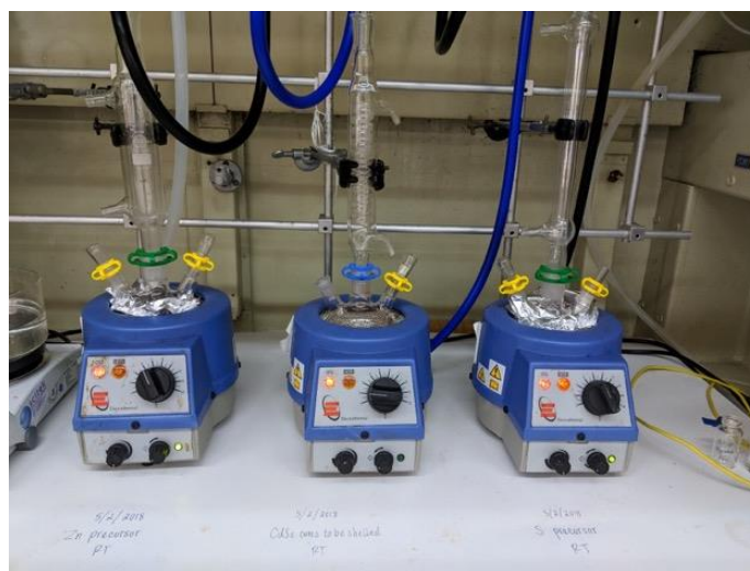
Figure 7.2. Benchtop setup with the cores in the middle, leftmost is the Zn precursor, and rightmost S precursor.
