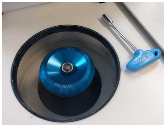
Figure 6.19. The cap was screwed on afterwards tightly using the hand tool before running the centrifuge.
