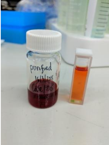
Figure 7.12. The CdSe/ZnS after purification deposited into chloroform before optical characterization.
