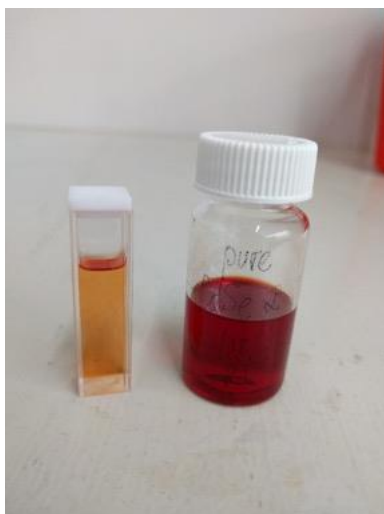
Figure 6.27. The 60 seconds reaction time mixture is now miscible with chloroform.
