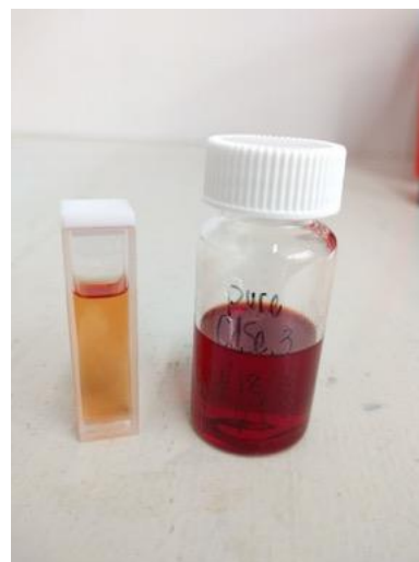
Figure 6.28. The 75 seconds reaction time mixture is now miscible with chloroform.
