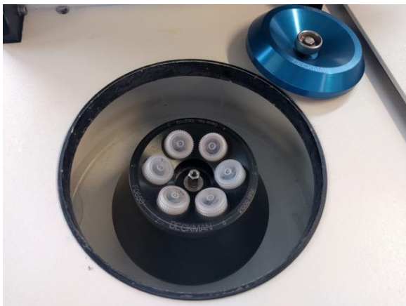
Figure 6.18. All 6 Falcon centrifuge tubes loaded into the benchtop centrifuge.
