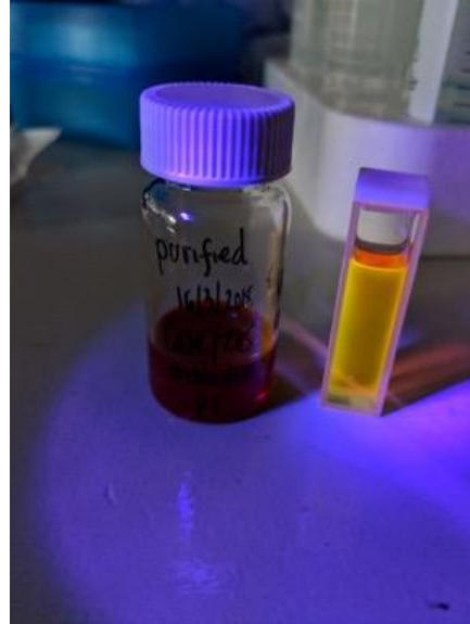
Figure 7.13. A bright orange fluorescence for the CdSe/ZnS under a 395 nm UV source.
