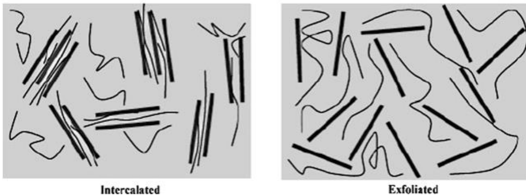
Figure 1.6. Nanoclays must be surface treated to transition from the intercalated to exfoliated state to maximize dispersion and performance increase in the nanocomposite [10] .
