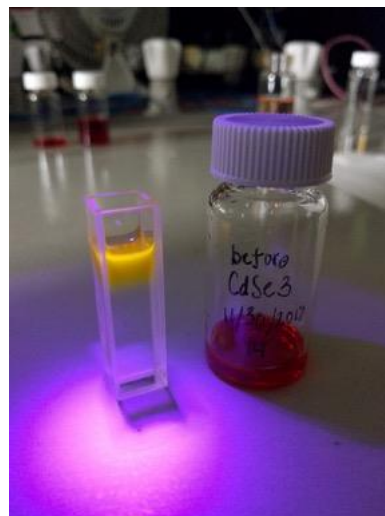
Figure 6.12. Quantum dots fluoresce under a 395 nm UV source, verifying they were synthesized correctly.
