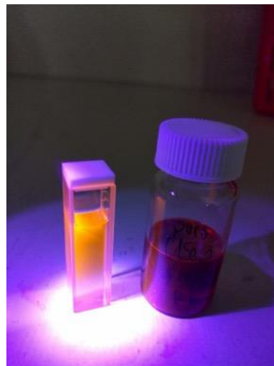
Figure 6.31. The 75 seconds batch fluoresces a bright orange color.
