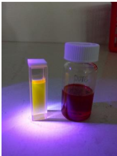
Figure 6.30. The 60 seconds batch fluoresces a deeper yellow color.
