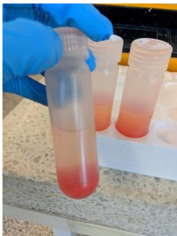
Figure 7.10. The quantum dots readily separated from the solvents even before centrifuging the sample.
