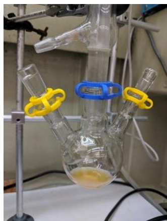
Figure 7.5. The zinc shelling precursor ready for alternating injection to generate the ZnS shells.
