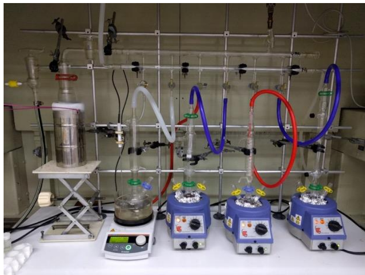
Figure 6.4. Scale up reaction where the three blue heating mantles are triplicate cadmium sources, and the selenium source is triple the amount in the oil bath.
