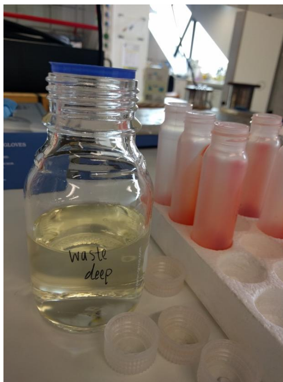
Figure 6.21. The first supernatant was very yellow, indicating collection and purification of raw mixture from impurities.
