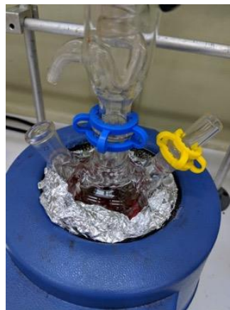
Figure 7.4. After 1 hour of allowing the chloroform to escape, the volume of the mixture is less than before.
