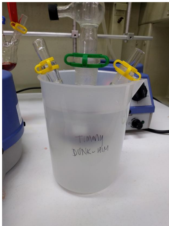
Figure 6.5. The reaction flask is quenched in a cold-water bath to stop the cores from growing too large.
