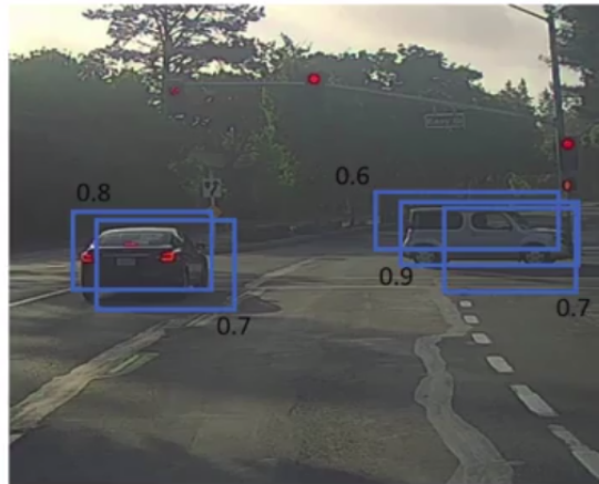
Figure 2.17: Detection without Non-Max Suppression [27]
