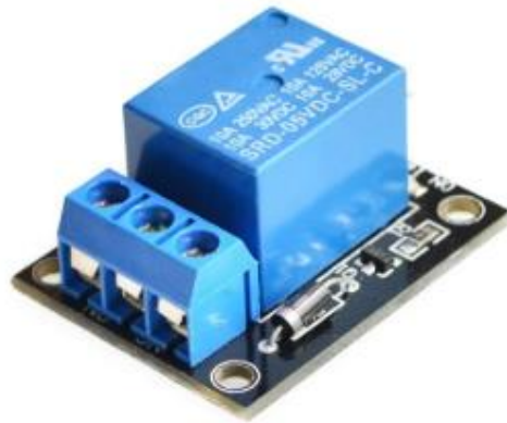
Figure 4-6: Tolako 5V Relay Module
