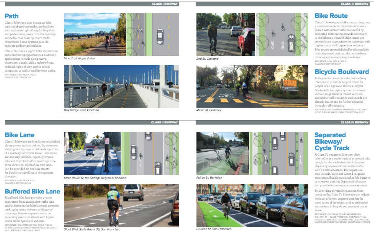
Figure 2: District 4 Bikeway Classifications of Class I-IV Bikeways to follow for the SHS [Caltrans District 4: A Guide to Bikeway Classification]
