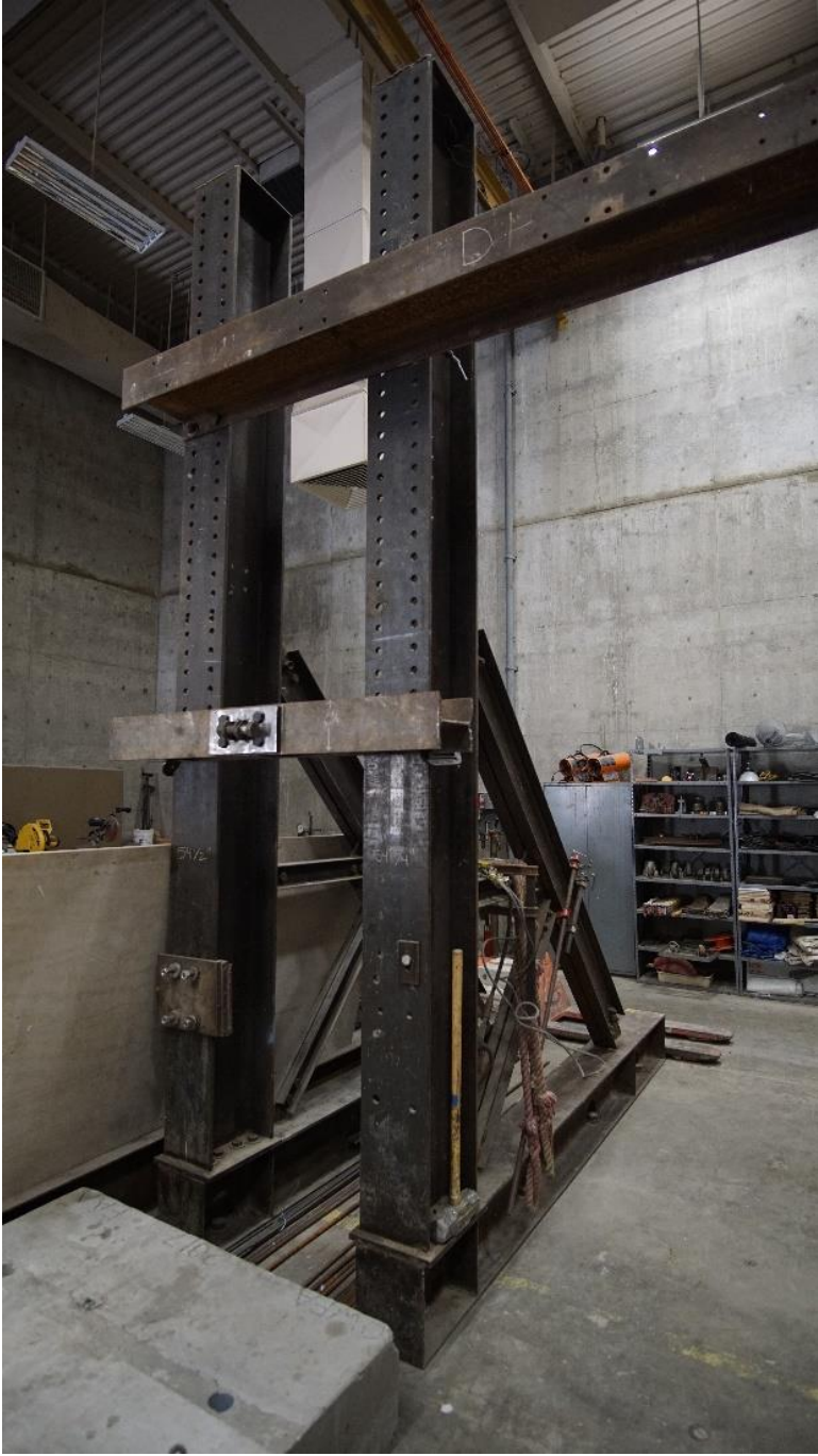
Figure 12: Front Right View of Reaction Frames
