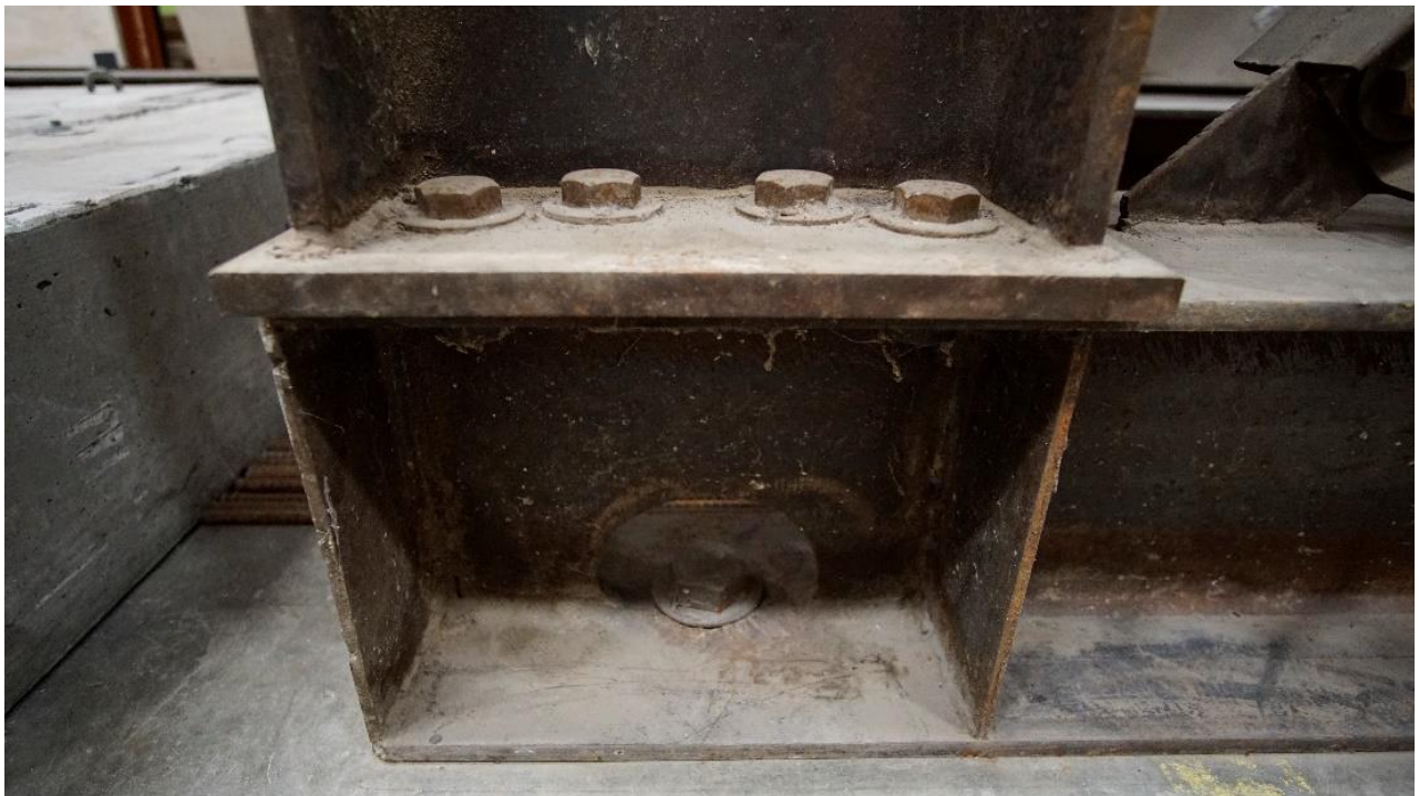
Figure 25 : Reaction Frame Column to Floor Beam Connection
