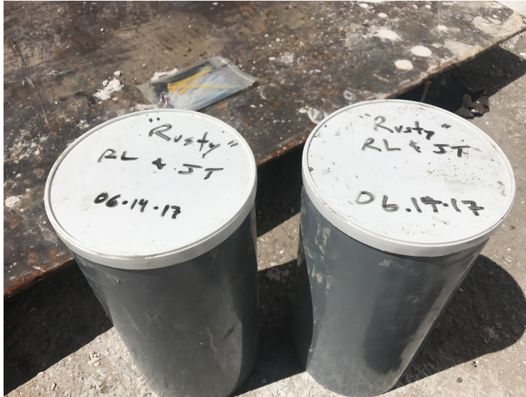
Figure 17: Concrete Cylinders for Compression Tests
