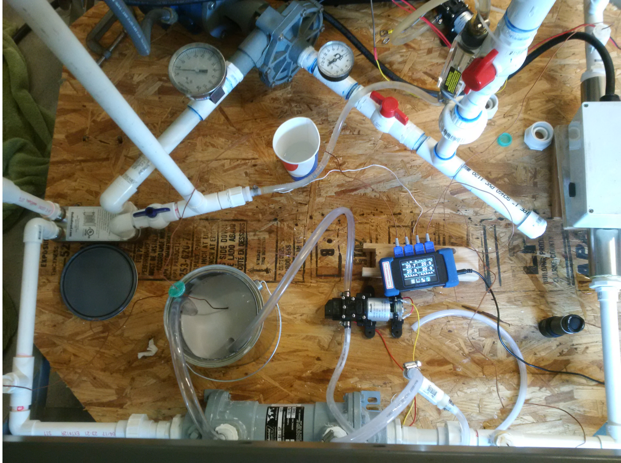
FIGURE 16 TOP DOWN VIEW, SHOWING BRAZED PLATE ON LEFT, TWO PUMPS, EXTERNAL PCM RESERVOIR.
