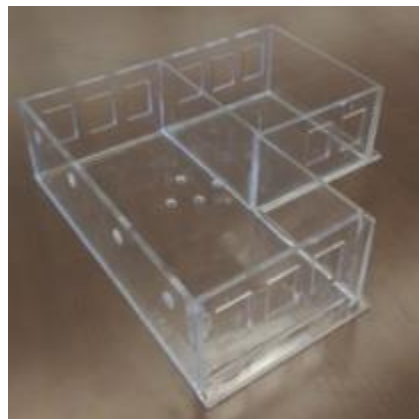
Figure 16. Wind Tunnel Model without Roof.
