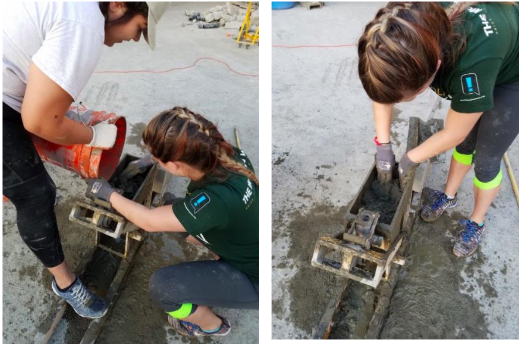
Figure 26. Cal Poly students pouring and pressing the cement mixture.
